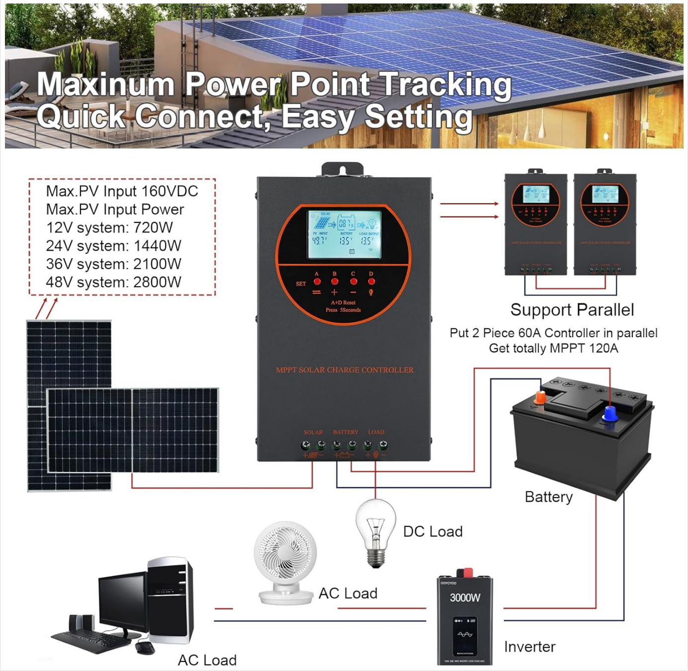
Figure 5.2: Illustrative wiring diagram showing connections from solar panels to the controller, then to the battery, and finally to DC and AC loads via an inverter. This diagram also shows the possibility of connecting two 60A controllers in parallel for increased capacity.
