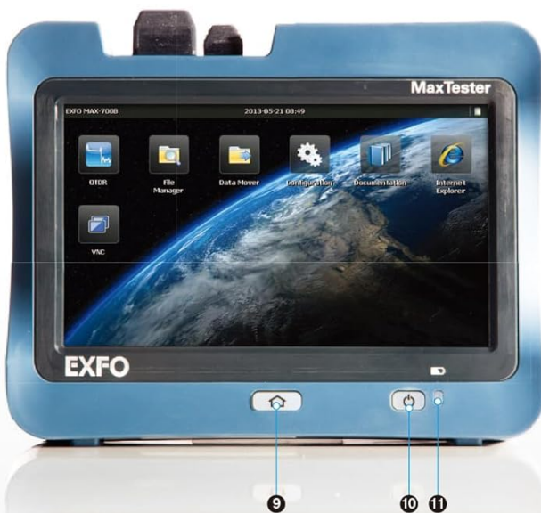
Figure 2.1: Front view of the EXFO MAX-710B OTDR with labeled ports and indicators.
