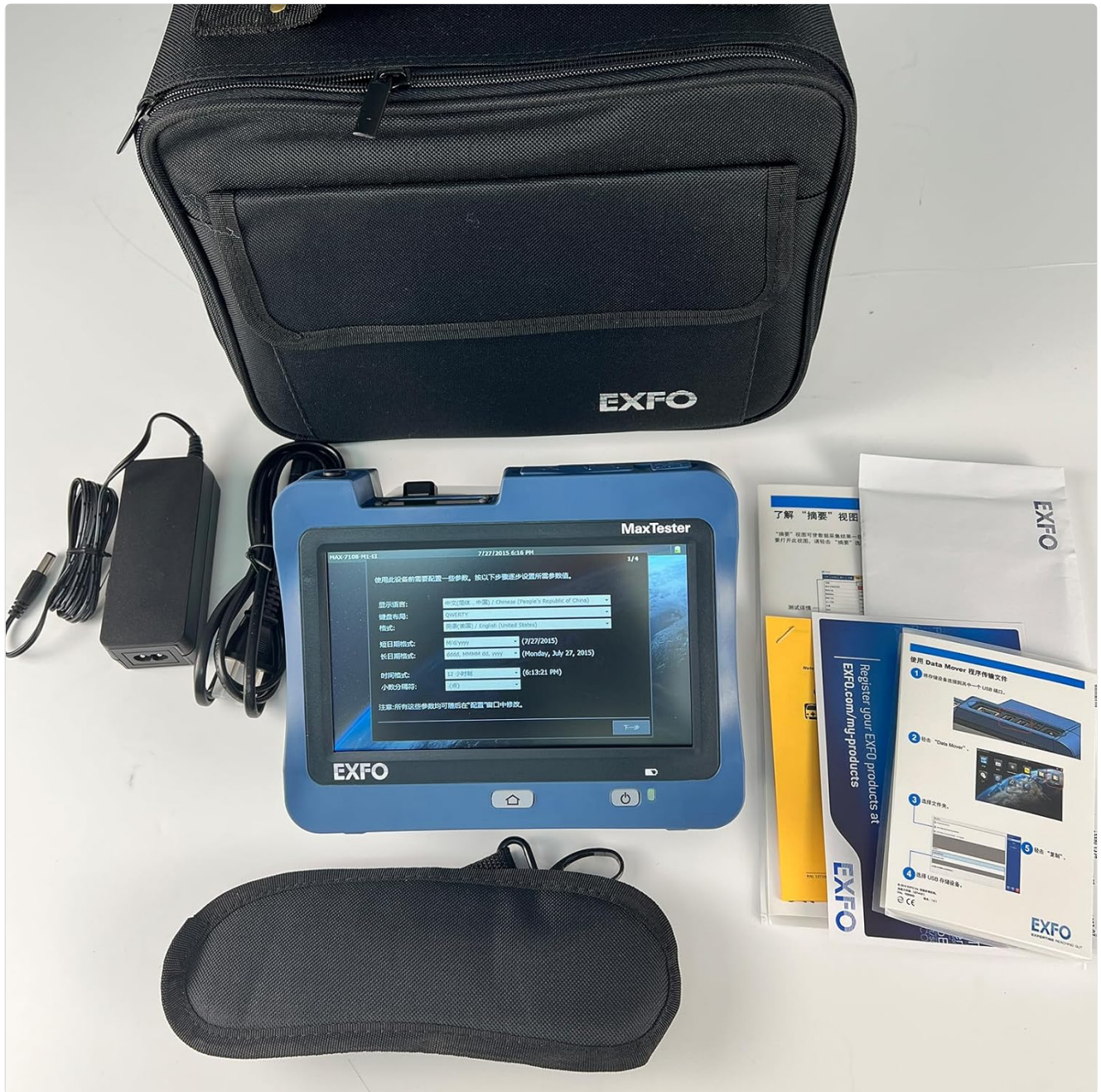
Figure 3.1: EXFO MAX-710B OTDR unit with typical accessories including charger, carrying bag, and documentation.
