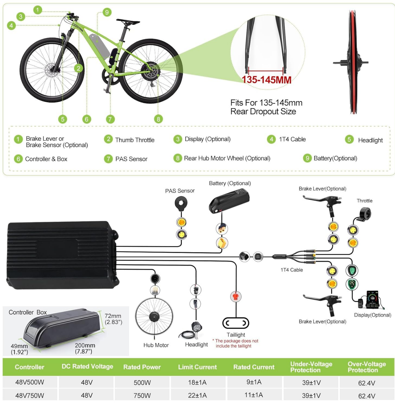
Image 5.1: Comprehensive wiring diagram showing the connection points for the hub motor, controller, battery, display, throttle, brake levers, PAS sensor, and headlight.
