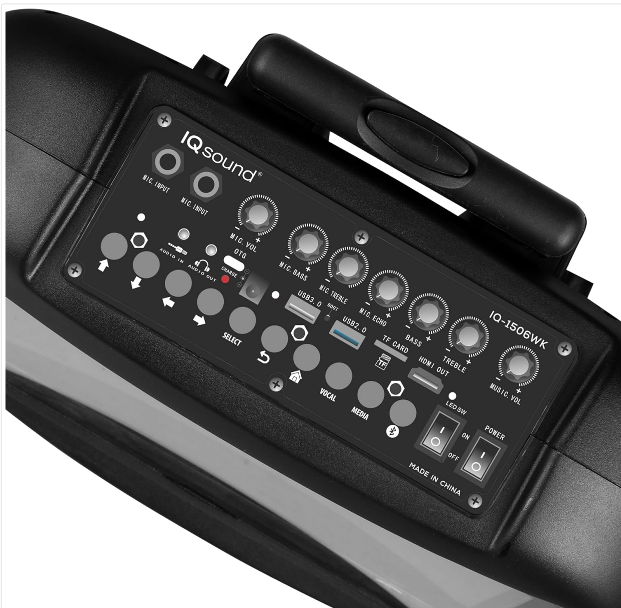
Figure 2: Detailed view of the control panel, showing knobs for Microphone Volume, Echo, Bass, Treble, and Master Volume, along with input ports for microphones, AUX, TF Card, USB, and HDMI Out.
