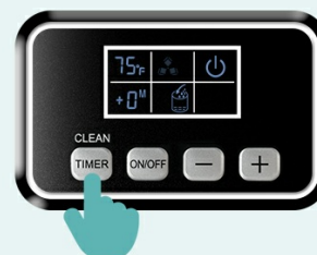
Figure 6.1: Instructions for initiating the 90-minute automatic cleaning cycle by holding the 'CLEAN' button for 5 seconds.
