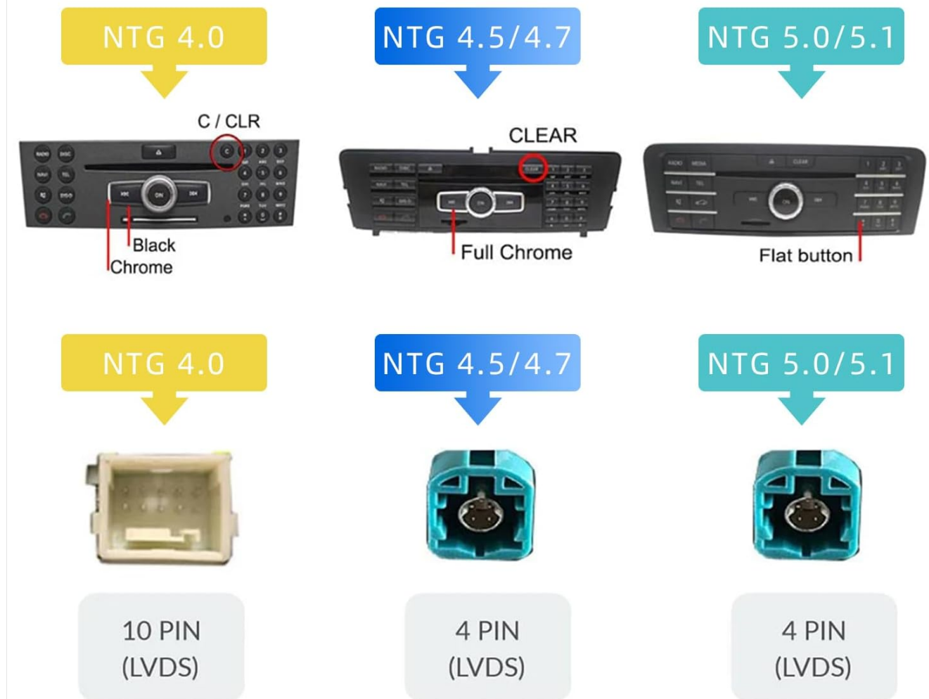
Figure 2: Visual guide for identifying Mercedes-Benz NTG 4.5/4.7 systems based on control panel appearance and LVDS connector type (4 PIN).
