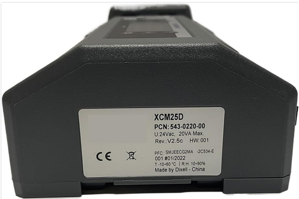
Figure 3.2: Side view of the ZDKOPCVR Unit Controller XCM25D, featuring a white product label. The label displays important information such as "XCM25D", "PCN: 543-0220-00", "U:24Vac, 20VA Max.", "Rev.:V2.5c", "HW:001", "T:-10-60°C", "R.H. 10-90%", and "Made by Dixell - China".
