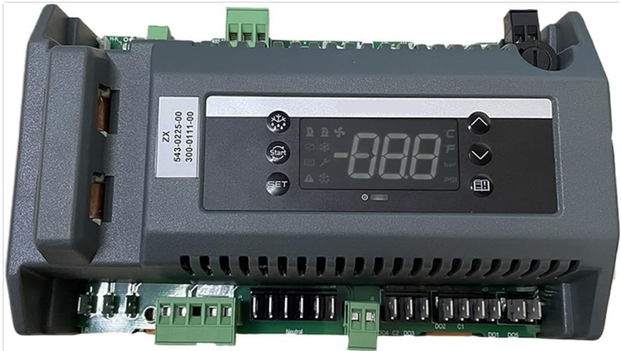
Figure 2.1: Front view of the ZDKOPCVR Unit Controller XCM25D. This image shows the main digital display, various indicator icons, and control buttons including 'Start', 'SET', 'Up', and 'Down' arrows. Several green terminal blocks are visible on the top and bottom edges of the unit.
