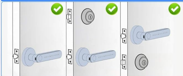
Figure 3: Door compatibility and handle reversibility for installation.
