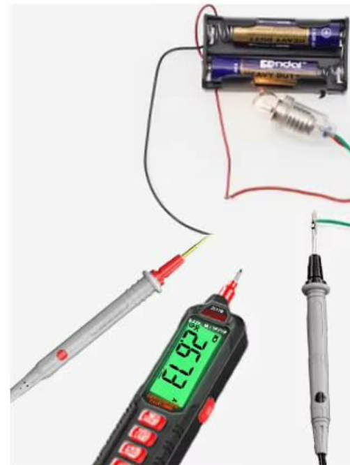
Measure current Connect the multimeter in series for circuit measurement A
