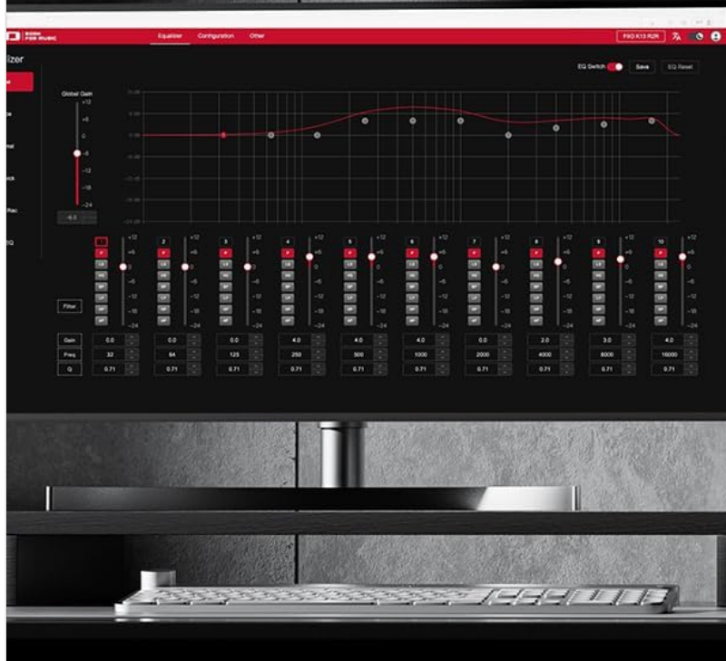
Figure 4: 10-Band High-Precision PEQ Interface. This image shows the graphical user interface for the 10-band Parametric Equalizer, demonstrating the ability to customize sound profiles across various frequency bands.
