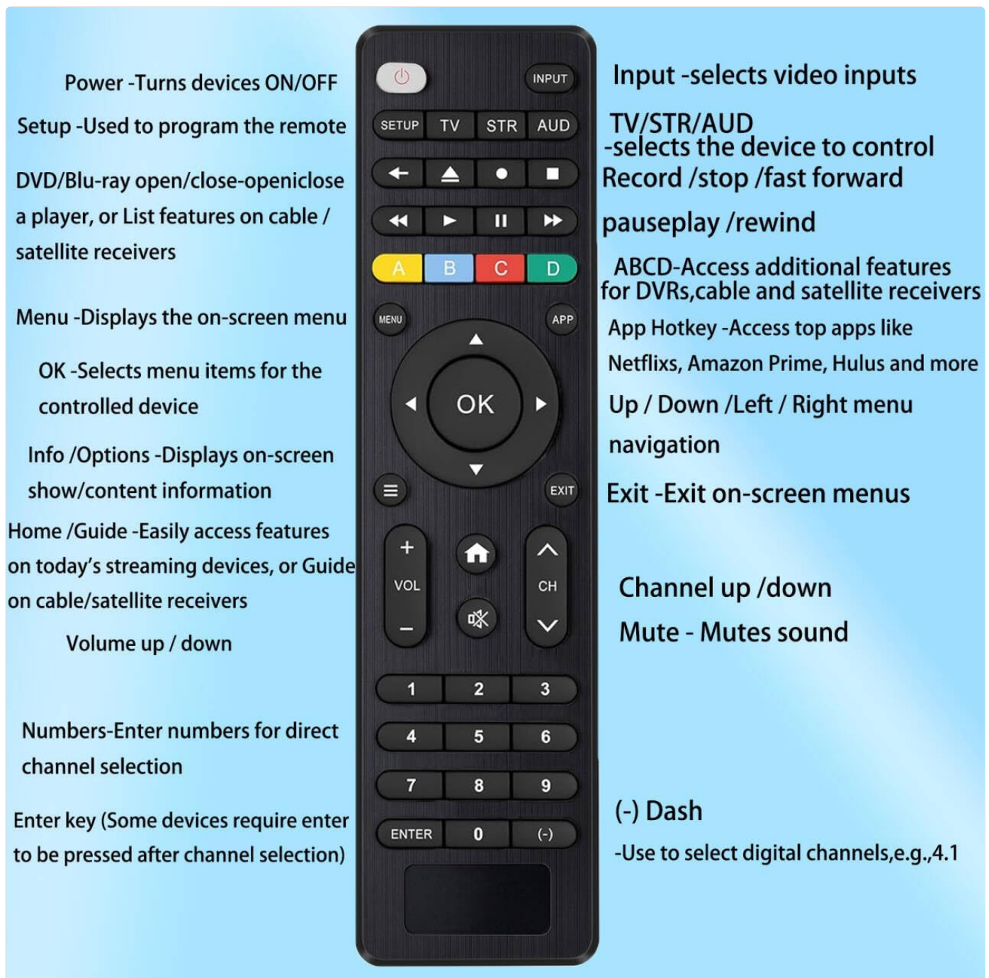
Image: Front view of the Pairtty Universal Remote Control with labels indicating the function of each button, such as Power, Input, Setup, TV, STR, AUD, navigation keys, volume, channel, number pad, and media playback controls.
