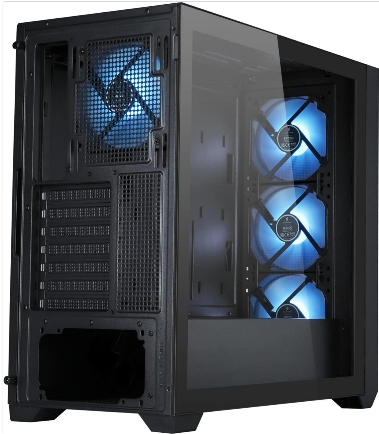
This perspective highlights the tempered glass side panel, allowing a clear view of the internal components. The rear 120mm A-RGB fan is also visible, contributing to exhaust airflow.
