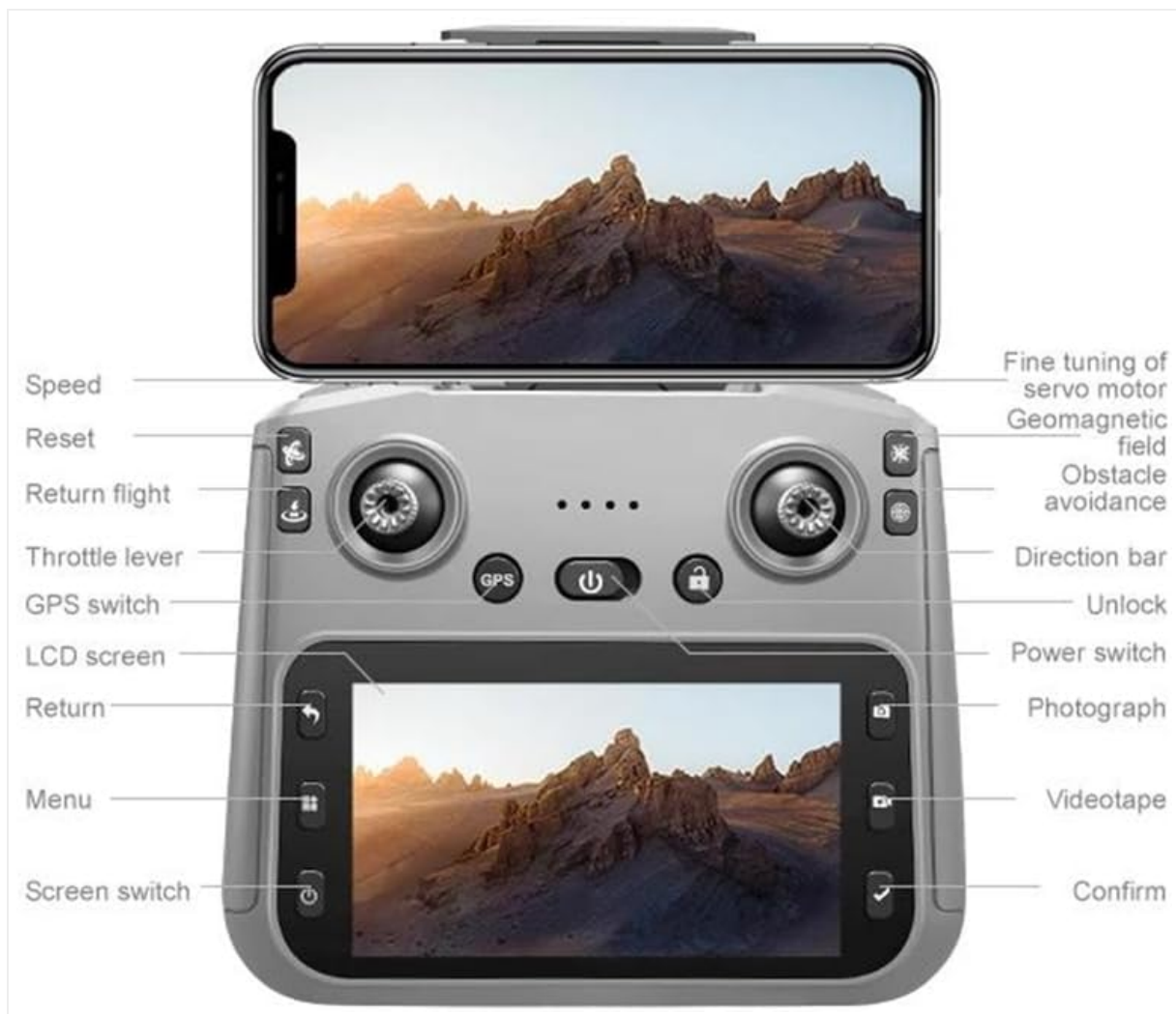
Figure 4.3: Remote Control Layout. This diagram illustrates the functions of each button and joystick on the remote control, including the integrated 5.6-inch display.
