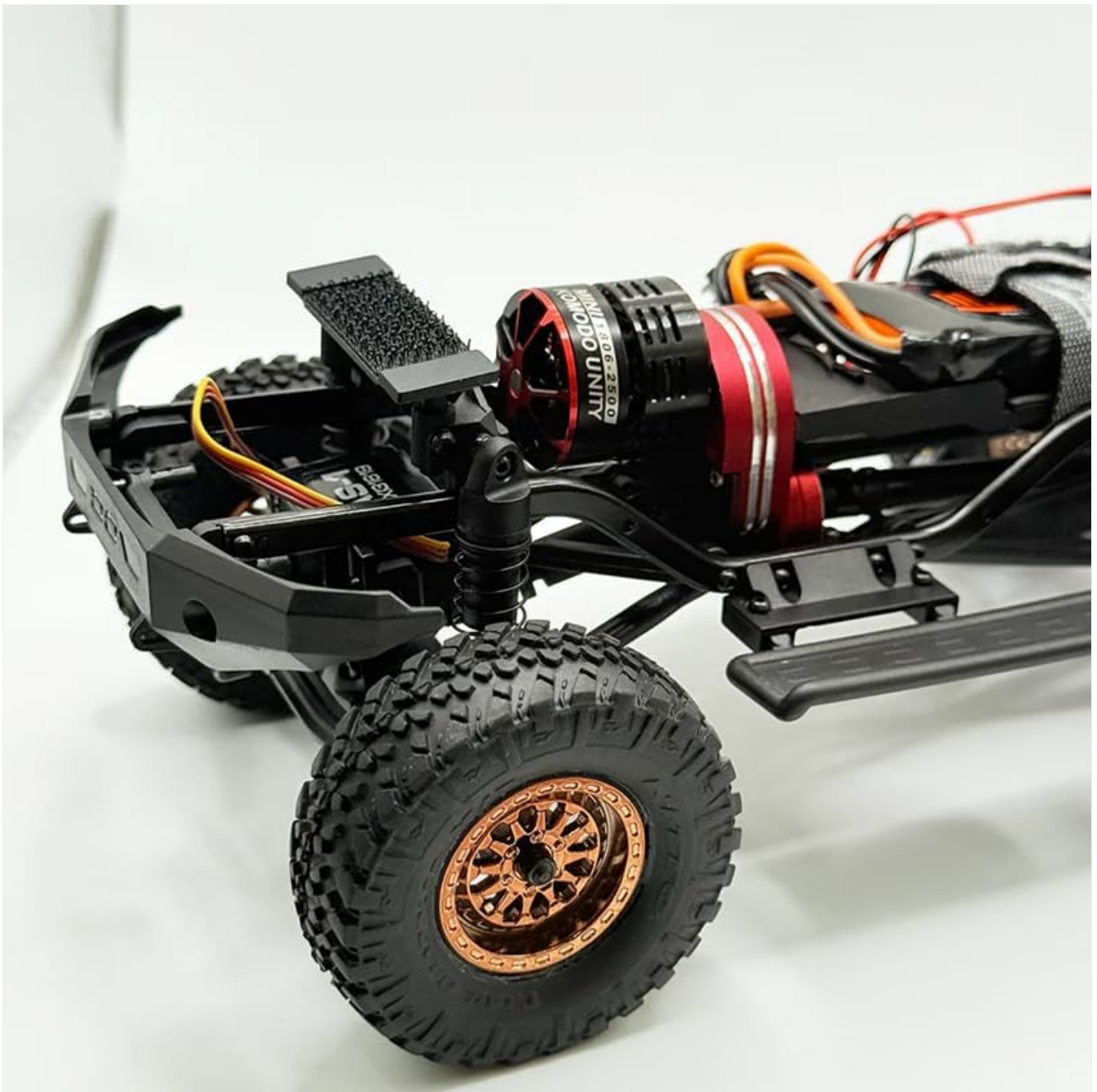
Image: The UNITYDRIVE Combo neatly installed within an Axial SCX24 chassis, demonstrating its compact integration and clean wiring.
