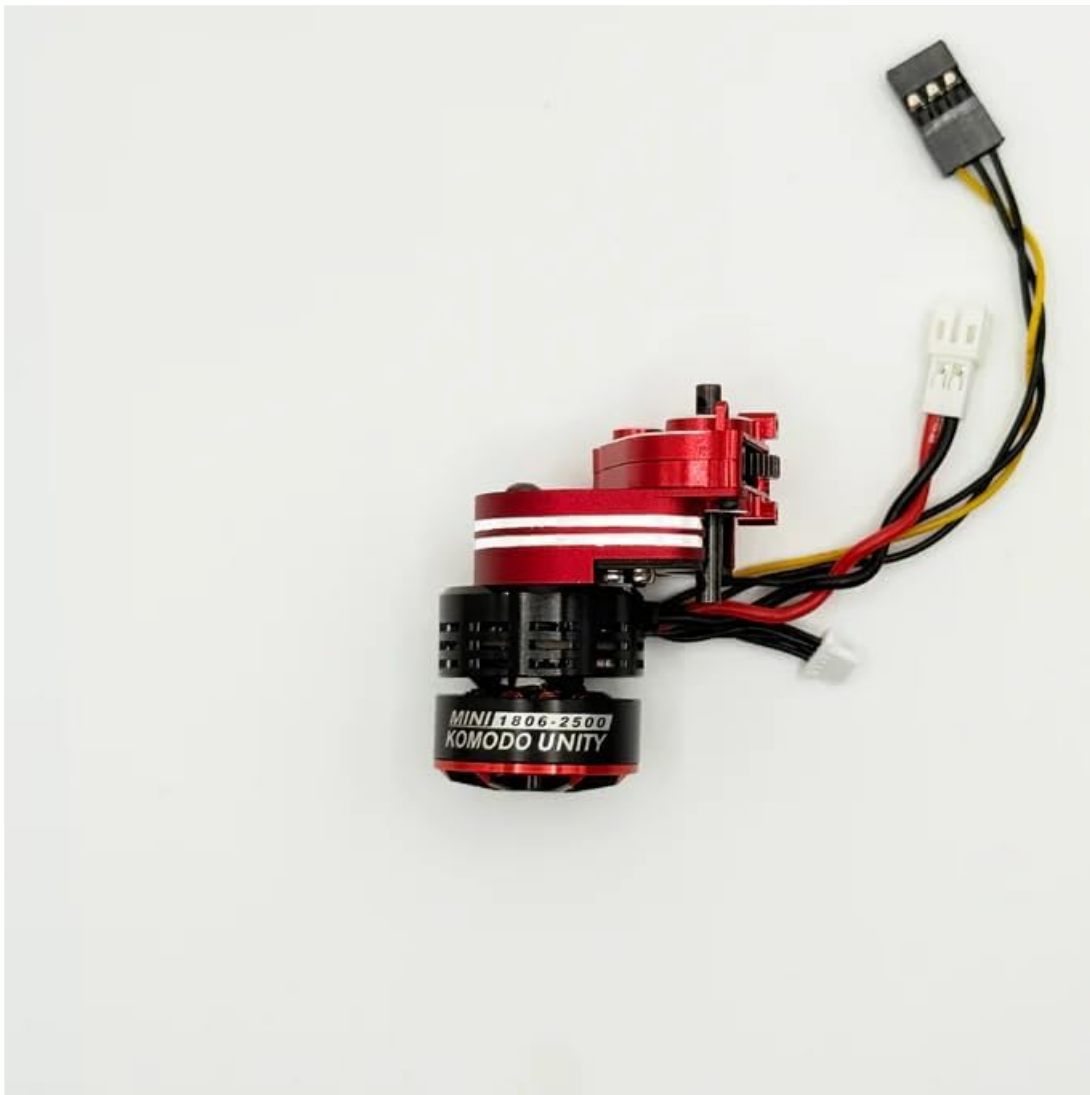
Image: The complete FURITEK UNITYDRIVE Combo, featuring the MINI KMD Unity 2-in-1 ESC/Motor connected to the Mini Stellar Transmission.
