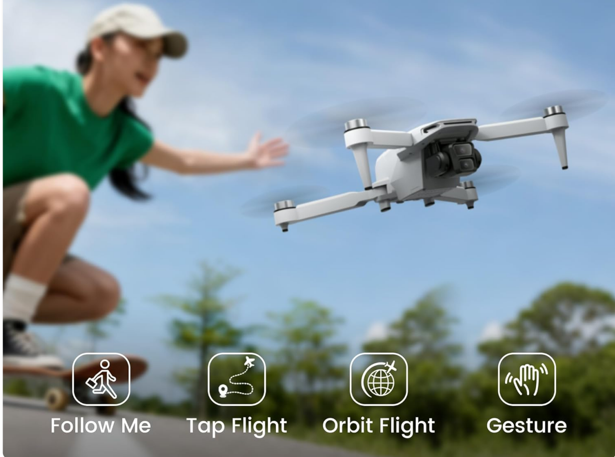
Image 5.2: The TizzyToy MT22 offers multiple smart flight modes, including Follow Me, Tap Flight, Orbit Flight, and Gesture Control, for enhanced creative possibilities.
