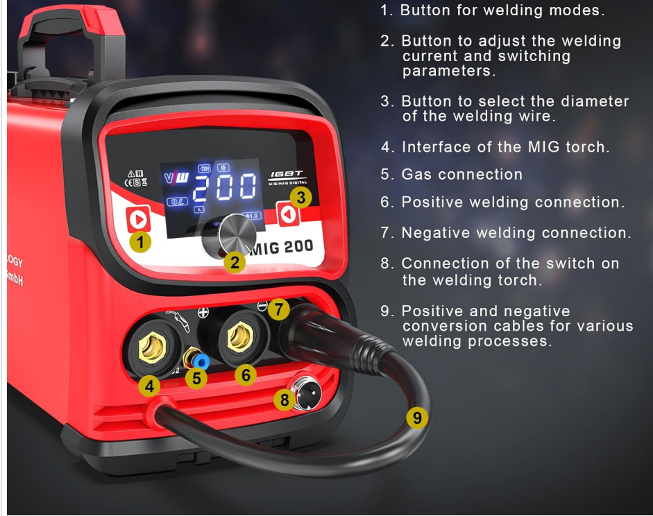
Figure 3: Front panel layout. Key components include (1) Welding mode button, (2) Welding current/parameter adjustment button, (3) Wire diameter selection button, (4) MIG torch interface, (5) Gas connection, (6) Positive welding connection, (7) Negative welding connection, (8) Welding torch switch connection, and (9) Positive and negative conversion cables.
