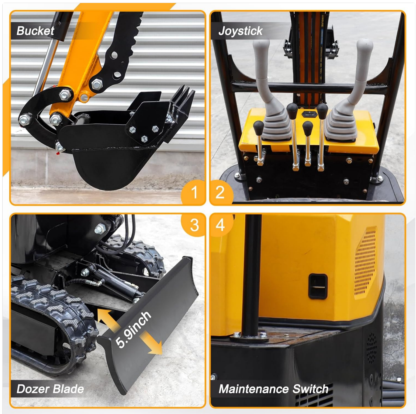
Figure 3: Detailed view of the bucket, joysticks for control, the dozer blade (adjustable up to 5.9 inches), and the maintenance switch.
