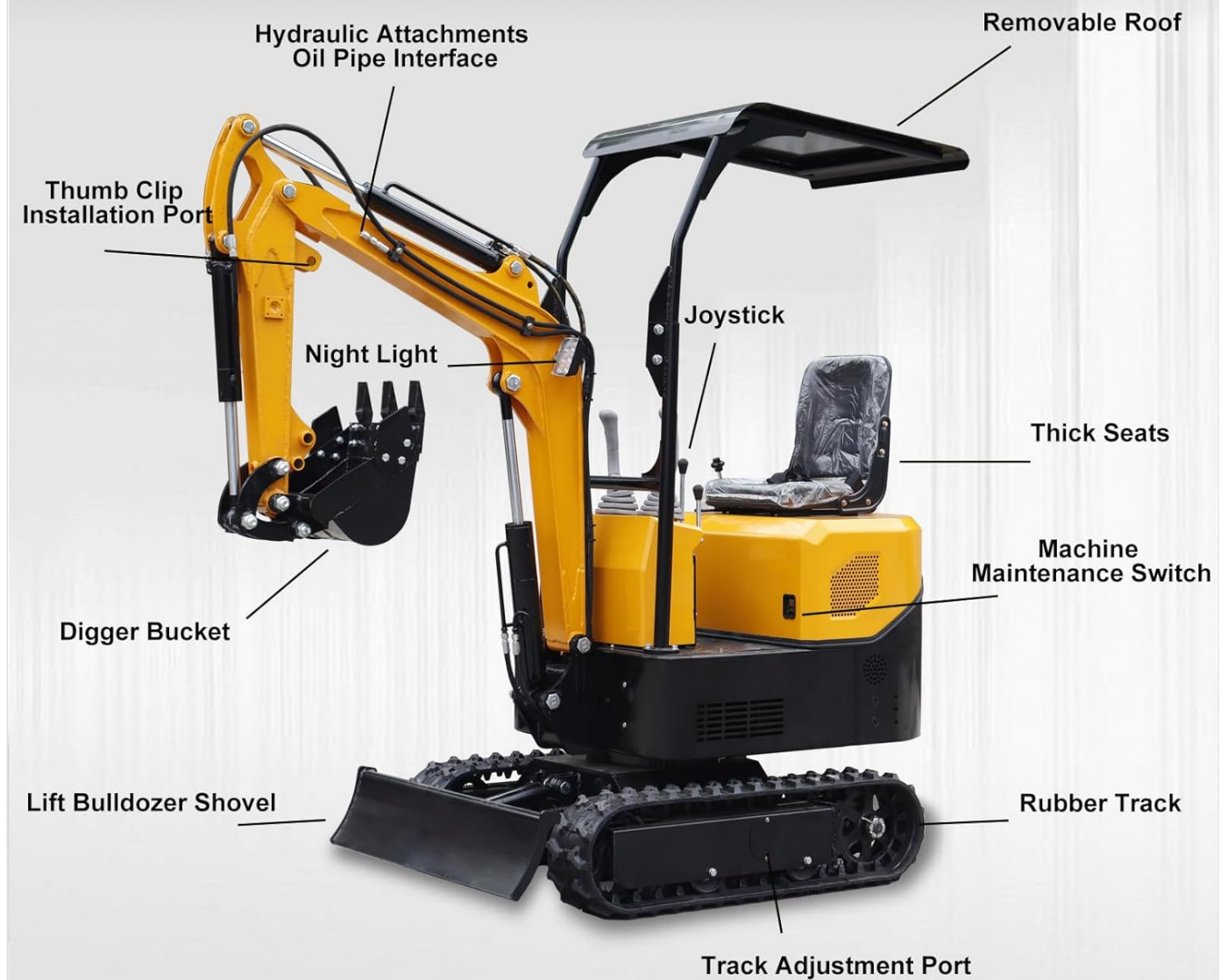
Figure 2: Excavator Structure and Controls. Key components include the digger bucket, joystick, hydraulic attachments oil pipe interface, removable roof, night light, thumb clip installation port, thick seats, machine maintenance switch, lift bulldozer shovel, rubber track, and track adjustment port.
