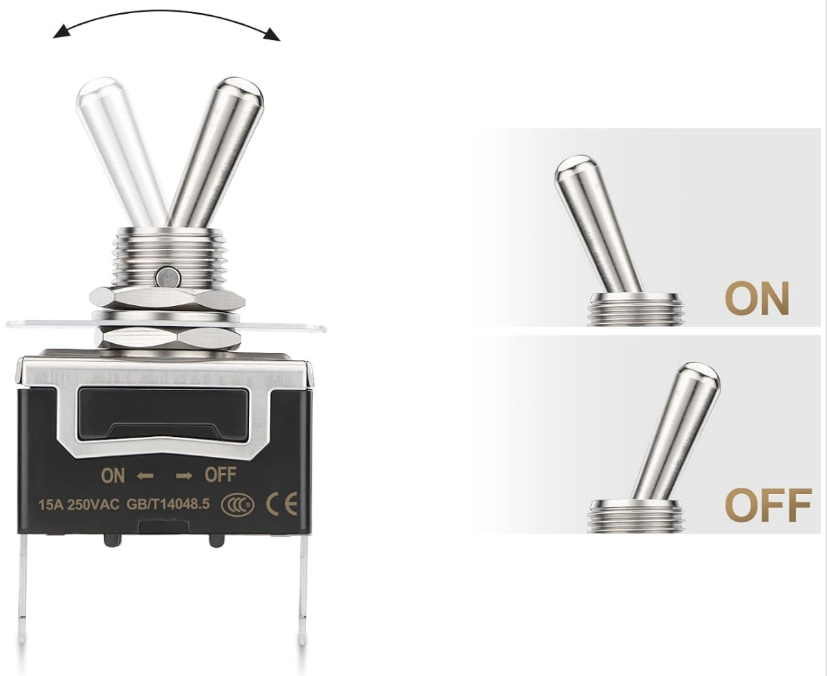
Image 6: SPST 2 Terminal Operation. This image demonstrates the ON and OFF positions of the toggle switch lever, clarifying its single-pole, single-throw functionality.
