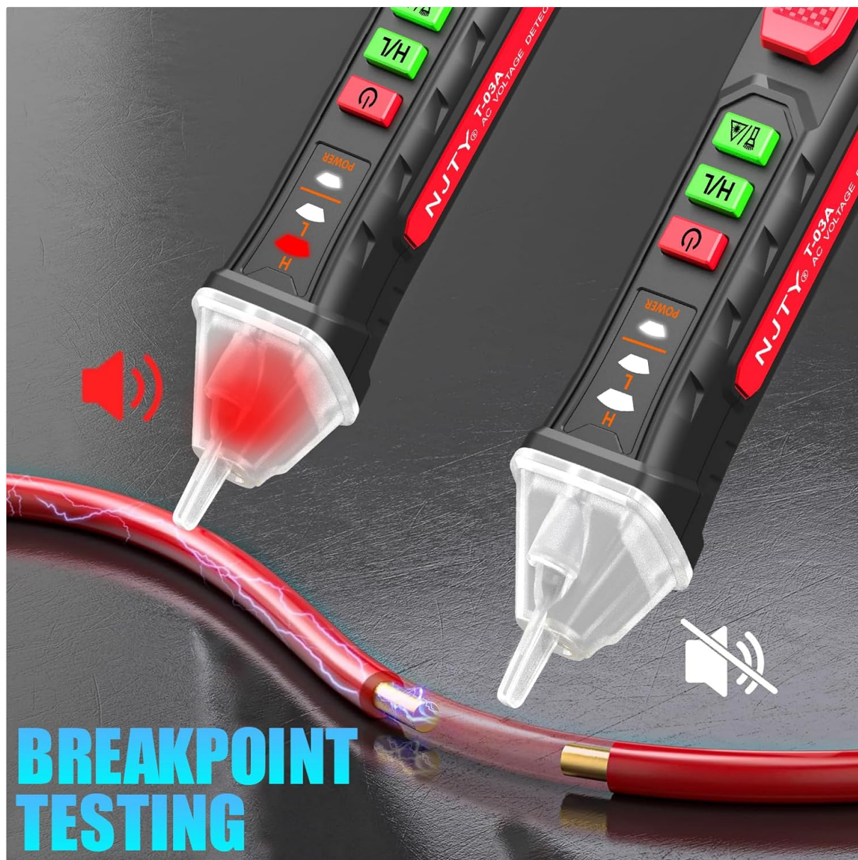
Image 6: Illustration of breakpoint testing. The tester indicates voltage on one side of a broken wire, and no voltage on the other side, pinpointing the location of the break.
