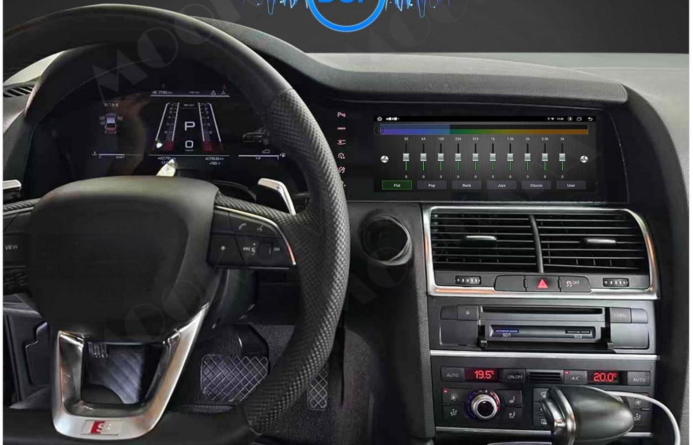
Image: The car radio display showing the 32-bit DSP equalizer interface, allowing users to adjust audio settings.
