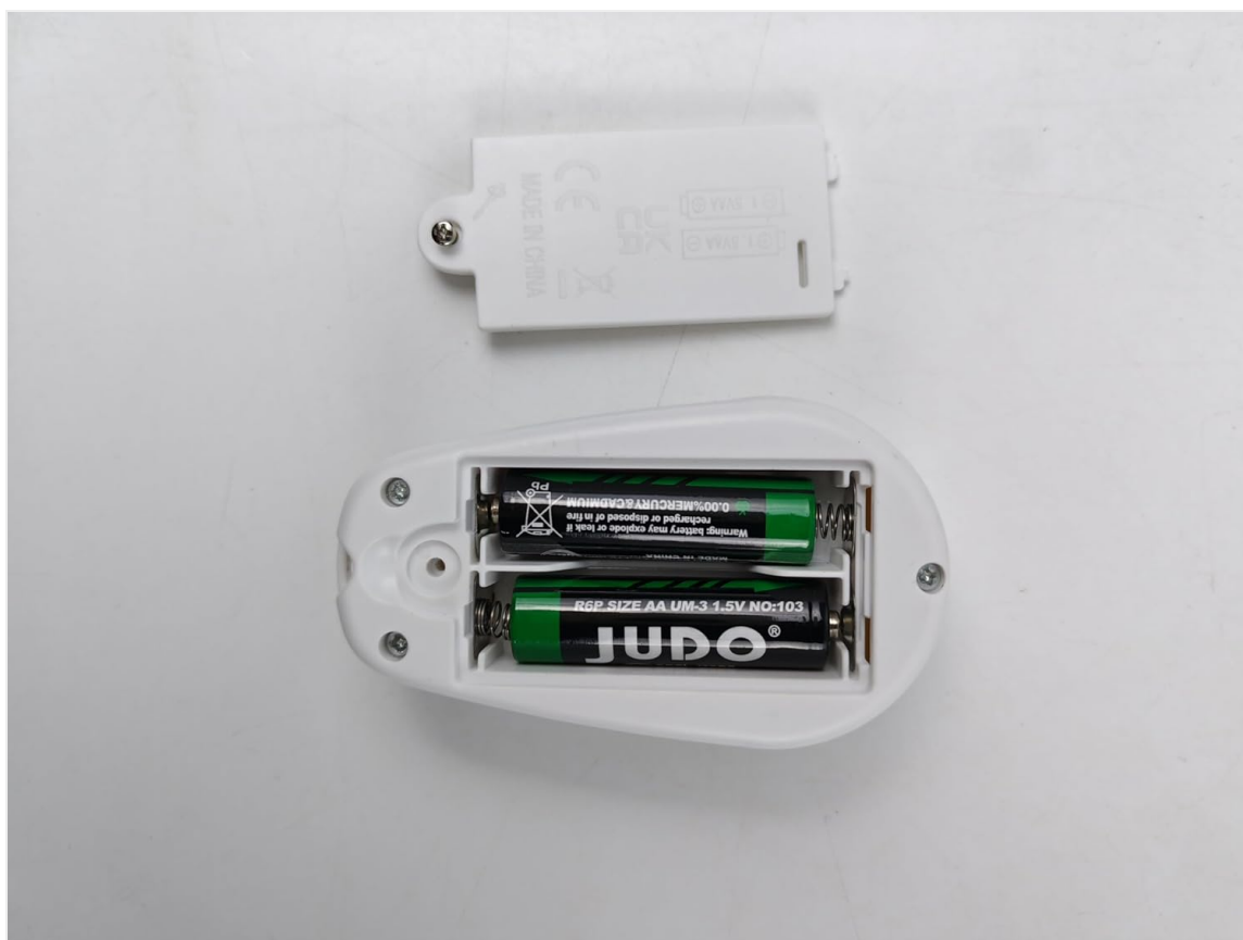
Image: The remote control with its battery cover removed, showing two AA batteries correctly installed.
