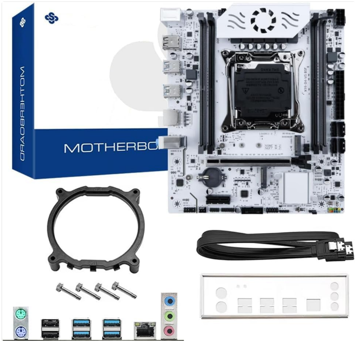
Figure 1: SOYO X99 BSF Motherboard and included accessories, including the I/O shield, SATA cable, and CPU cooler mounting bracket.
