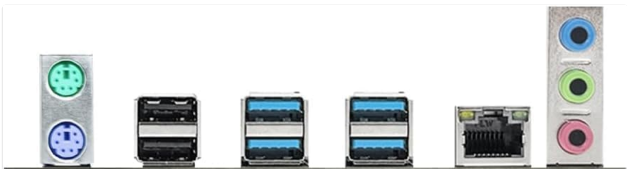
Figure 3: Close-up view of the rear input/output panel, showing PS/2 ports, USB 2.0 ports, USB 3.0 ports, RJ45 LAN port,
