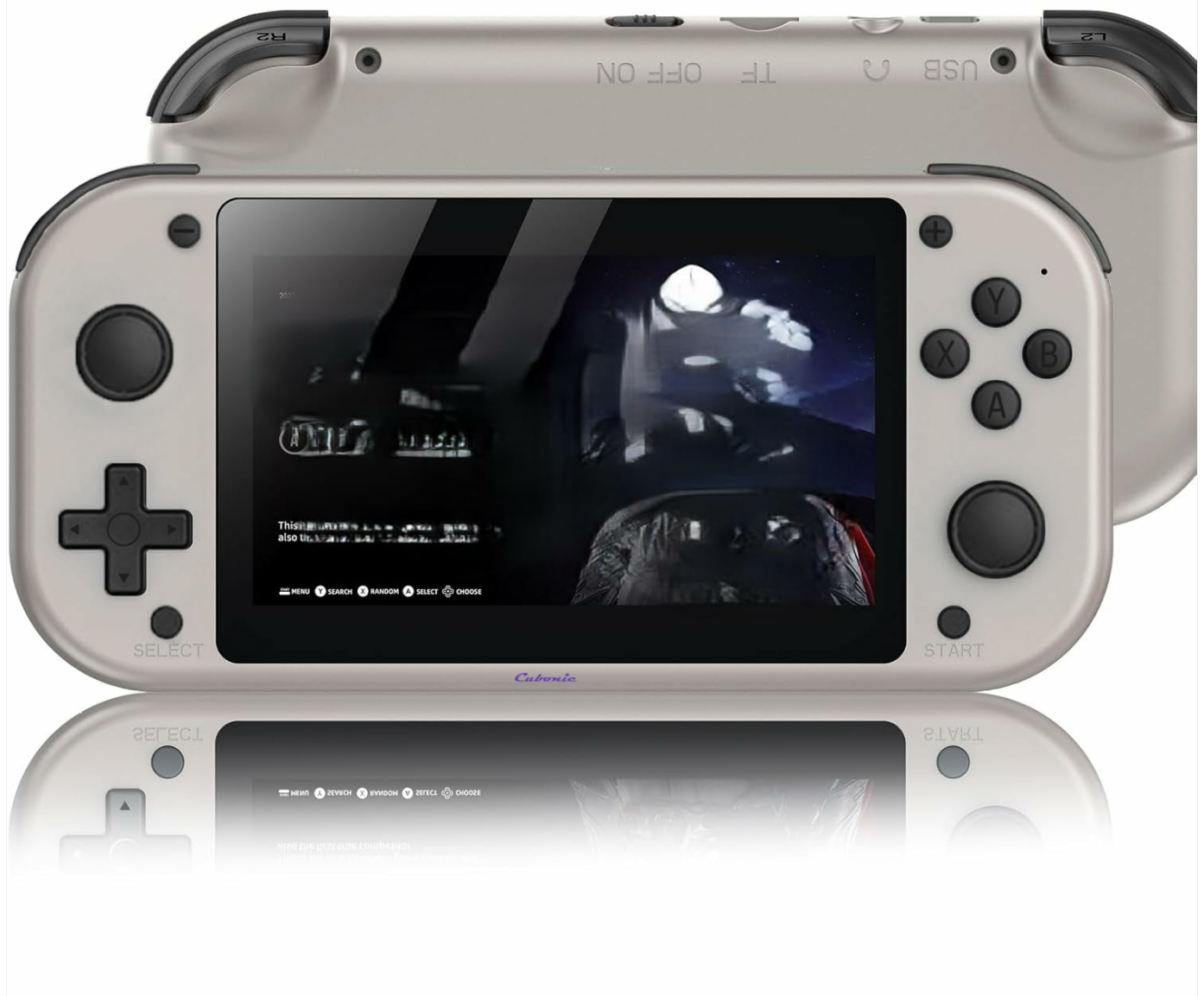
Image 2.3: Rear view of the console, highlighting the TF card slot and USB port.
