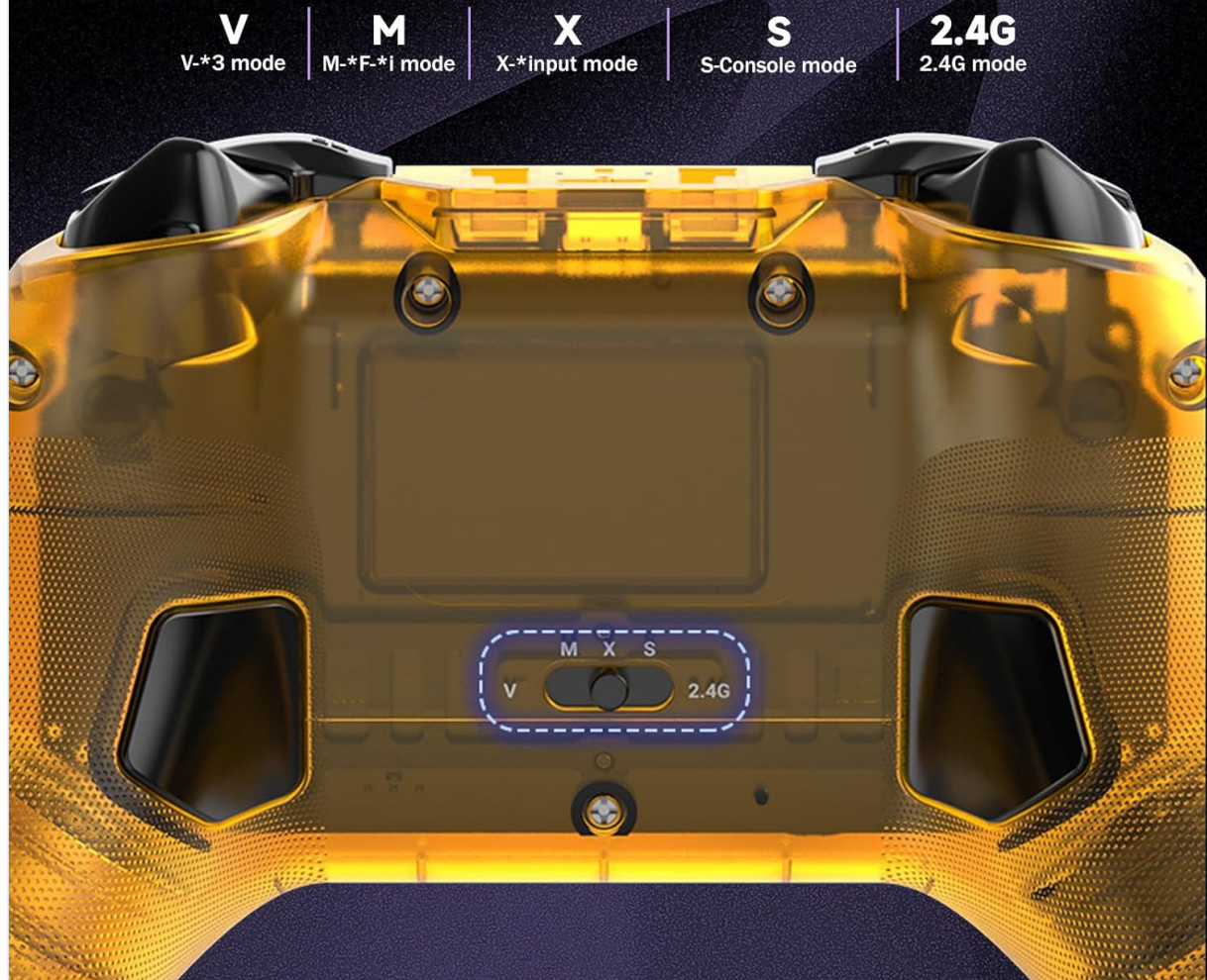
Image 3: Location of the 5 Modes Keys switch on the controller, indicating 2.4G, V, M, X, and S modes.
