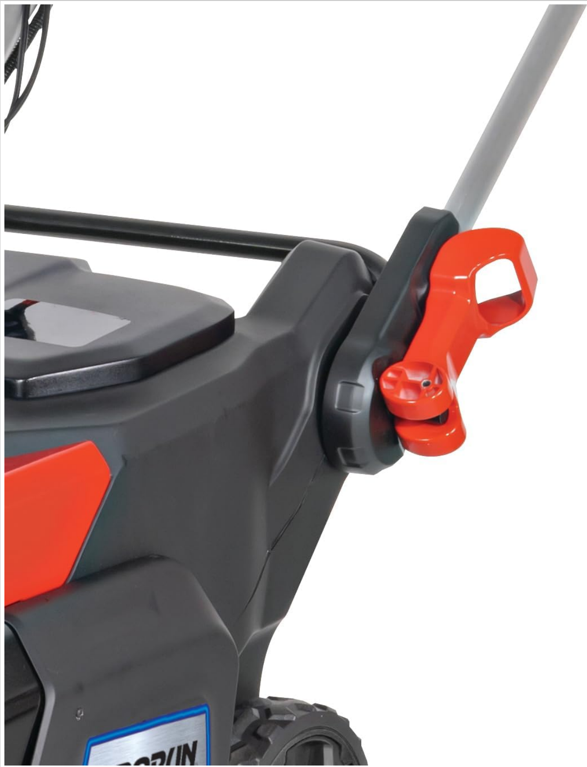
Image: A close-up of the handle release lever on the PRORUN snow blower, which facilitates folding the handle for compact storage and transport.
