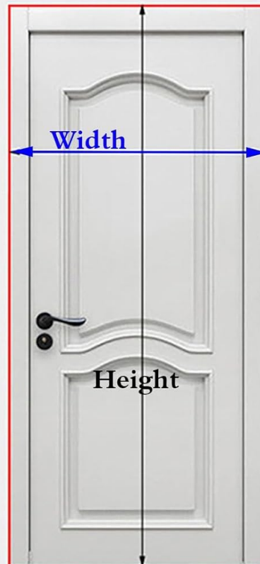
Figure 2: Visual guide for measuring door openings for both inside and outdoor mounting. Inside mounting requires measuring width and height at multiple points and using the minimum value. Outdoor mounting involves measuring the desired coverage area.
