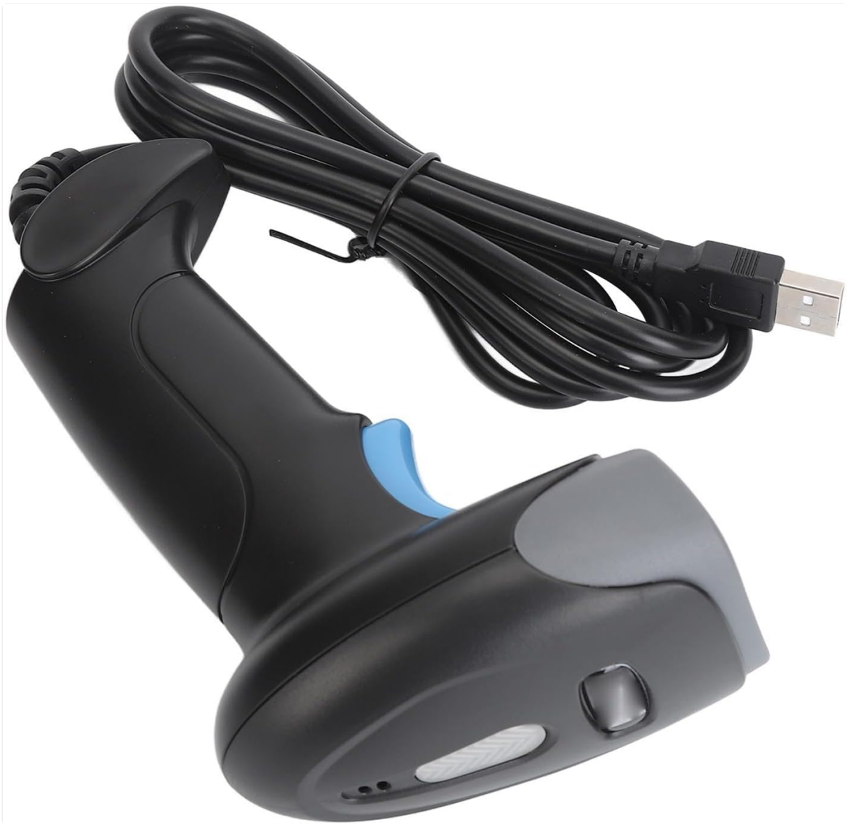
Figure 3: Side view of the scanner, showing the integrated USB cable.
