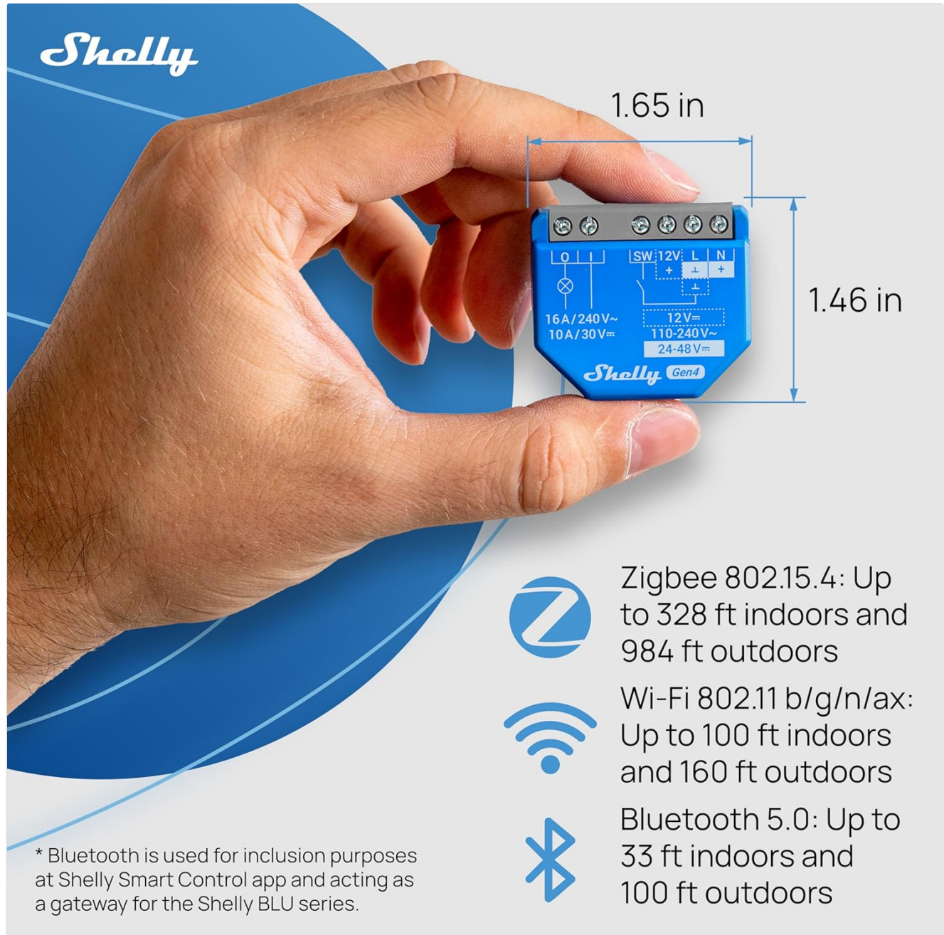
Image 4.1: Shelly 1 Gen4 showing dimensions (1.65 in x 1.46 in) and wireless connectivity ranges for Zigbee, Wi-Fi, and Bluetooth. The device features terminals for Line (L), Neutral (N), Input (I), Output (O), and Switch (SW). It also includes dedicated terminals for 12V DC and 24-48V DC power supply options, alongside the standard 110-240V AC input.
