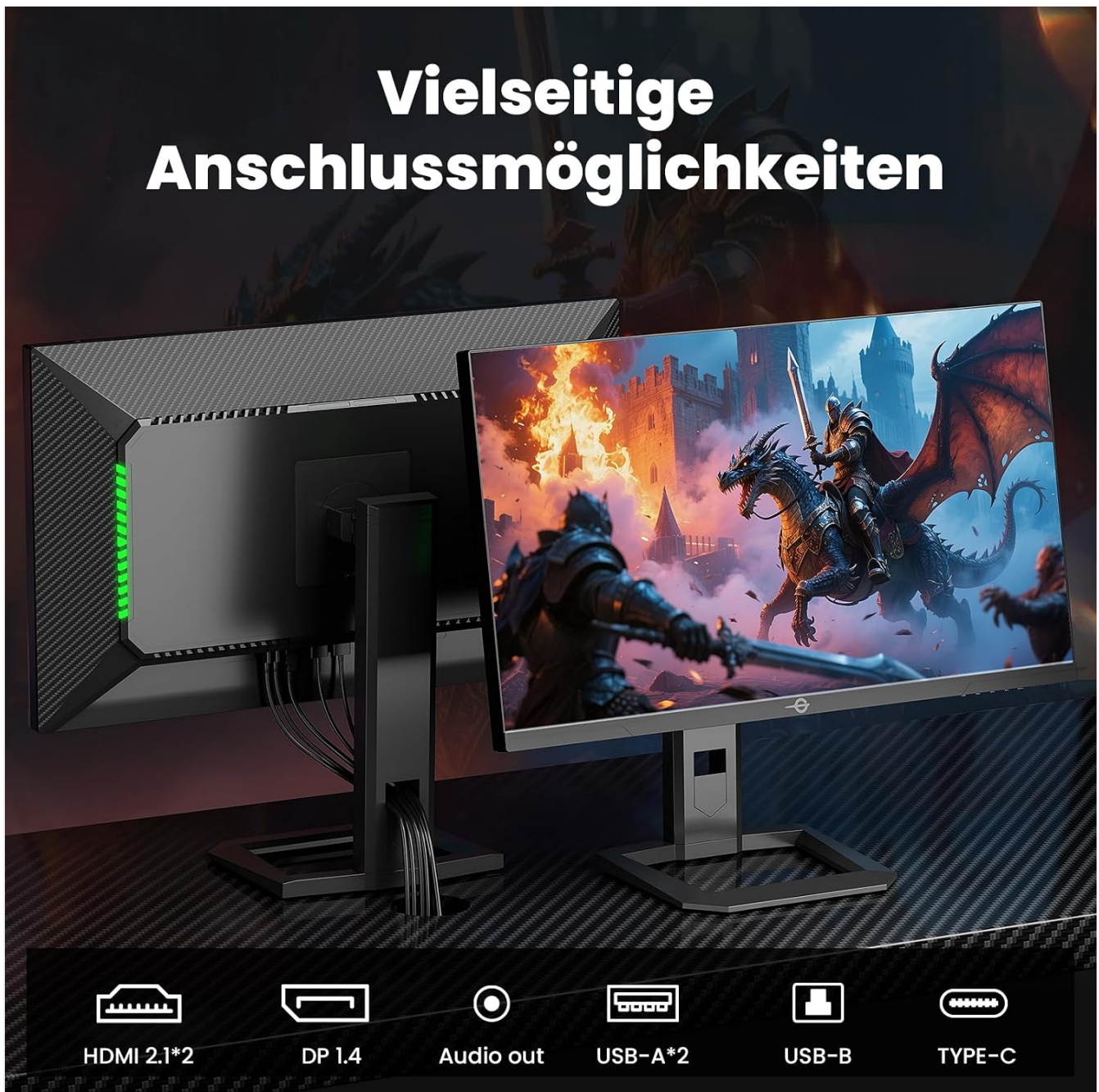
Image: Rear view of the TITAN ARMY P275MV Plus monitor, highlighting the HDMI 2.1 (x2), DisplayPort 1.4 (x1), USB-C (x1), USB-A (x2), USB-B (x1), and audio output ports. This illustrates the versatile connectivity options available.
