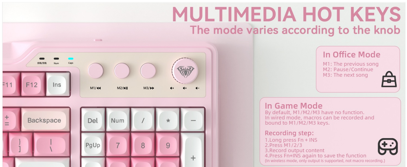
Image: Explanation of the multimedia hot keys (M1, M2, M3) and their functions in both office and gaming modes.
