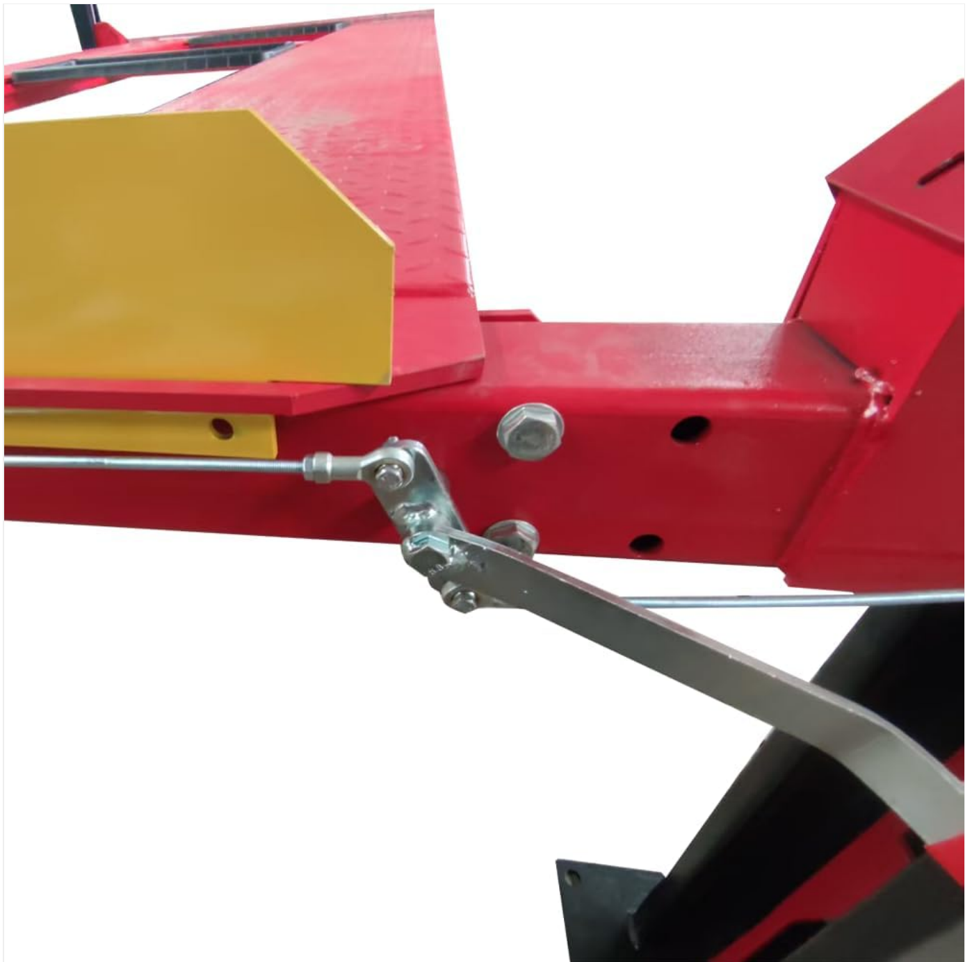
Figure 5.2: Detail of the lift's safety lock mechanism.
