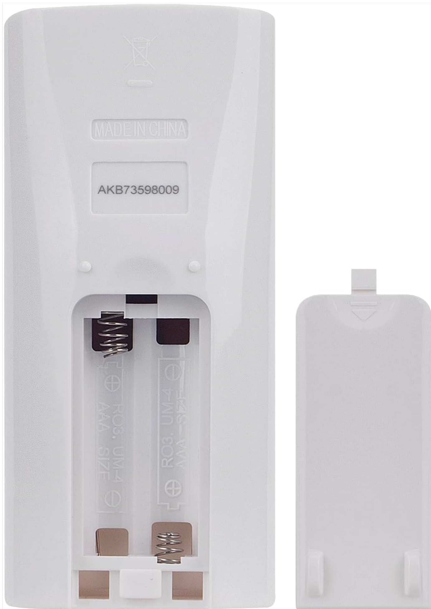
Figure 4: Open battery compartment, showing where to insert AAA batteries.
