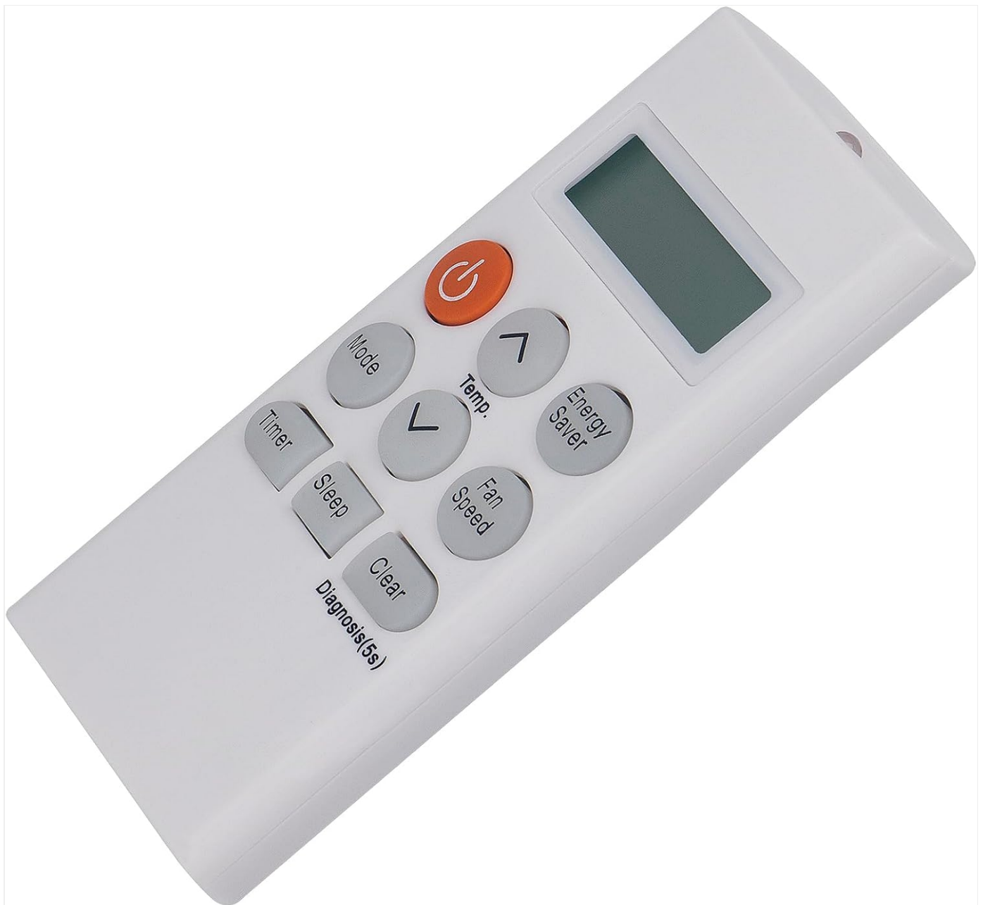
Figure 2: Angled view of the AKB73598009 remote control, highlighting button layout.
