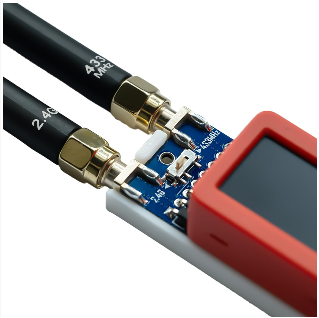
Image: Side view of the RF 2-in-1 module connected to the M5Stack StickC Plus, highlighting the antenna ports and the physical switch for selecting between 2.4GHz and 433MHz frequencies.
