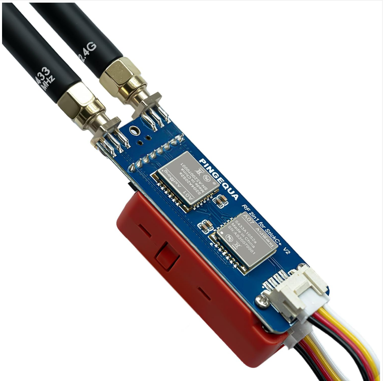
Image: Top view of the RF 2-in-1 module, highlighting the NRF24 and CC1101 chips, and the physical switch for selecting between 2.4GHz and 433MHz frequencies.
