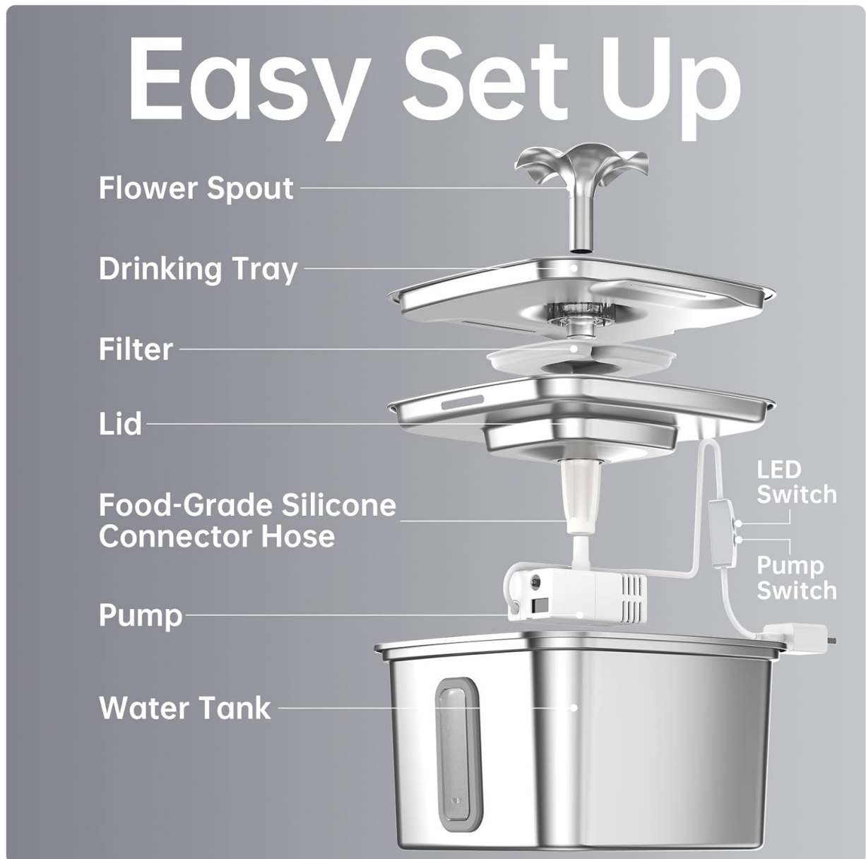
Image: Exploded view diagram showing the assembly order of the fountain components.
