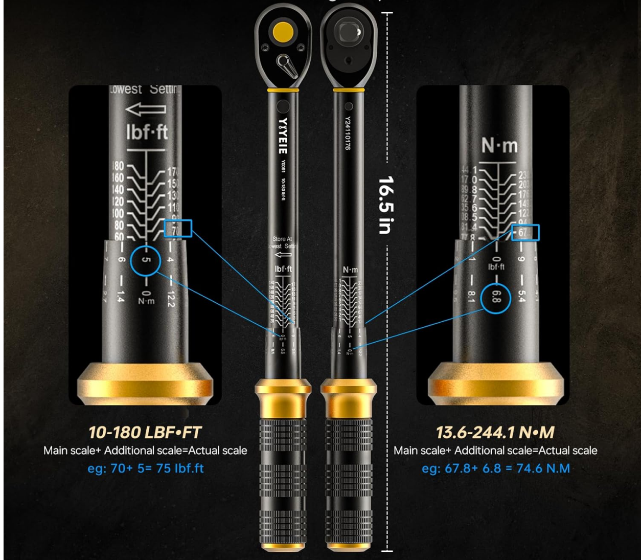
Image 3.2: Close-up view of the dual range scales (lbf-ft and N-m) on the torque wrenches, demonstrating how to read and set precise values.
