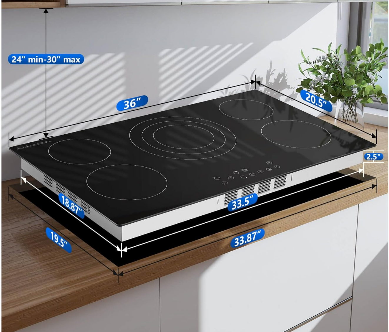
Figure 5: Cooktop dimensions and recommended cutout measurements for installation.
