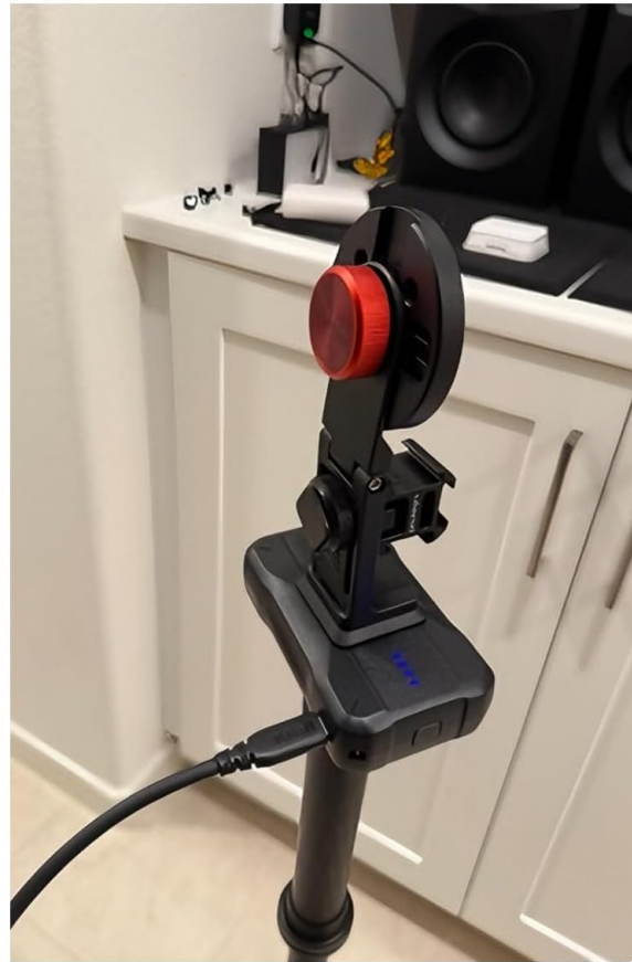
Image 5.1: The power bank can charge devices via its USB-A output or bidirectional Type-C port.
