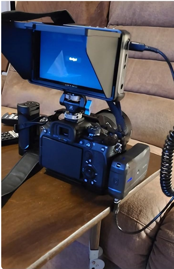
Image 5.1: The power bank can charge devices via its USB-A output or bidirectional Type-C port.
