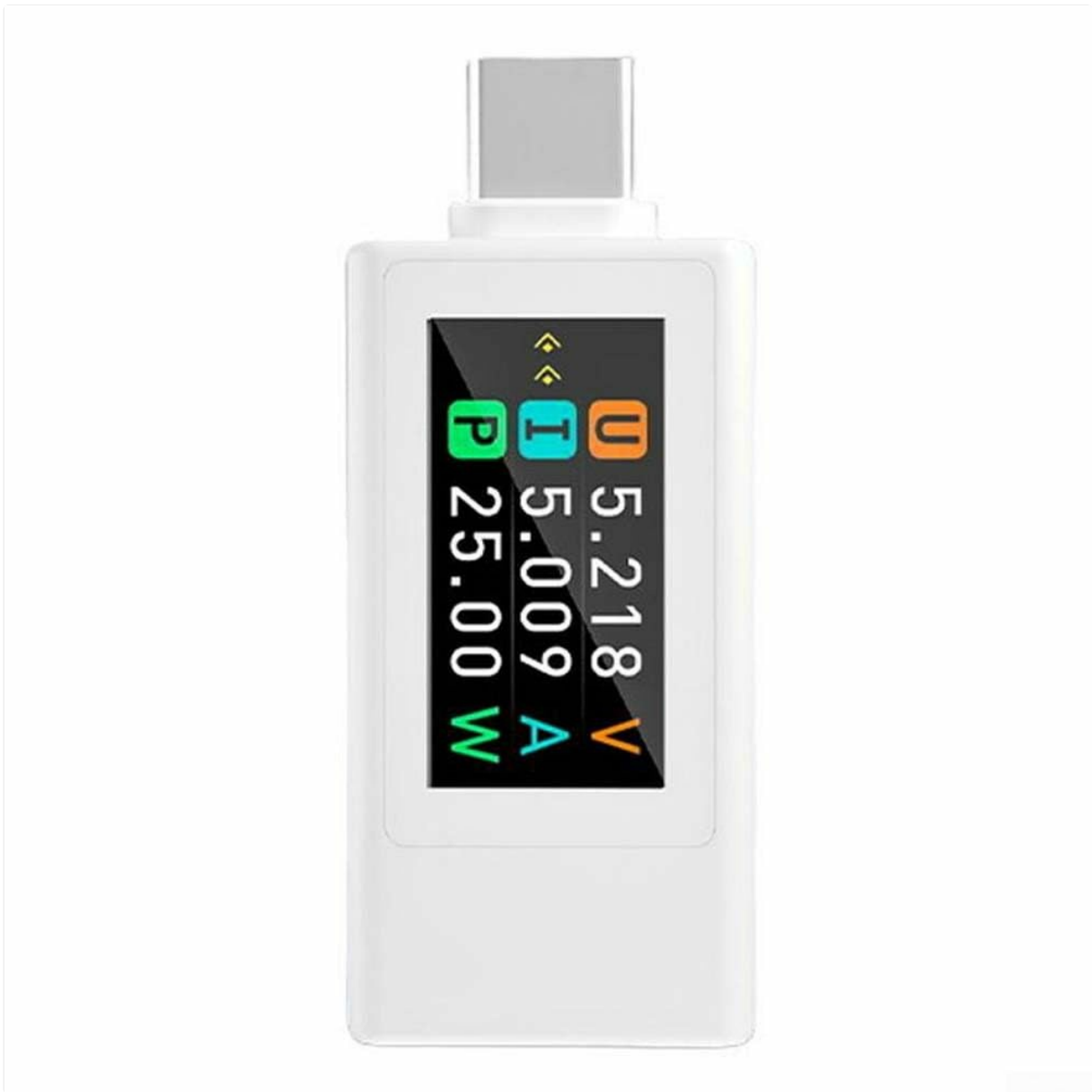
Figure 1: Front view of the Jurmy KWS-1902L Type-C Voltage and Current Tester.
