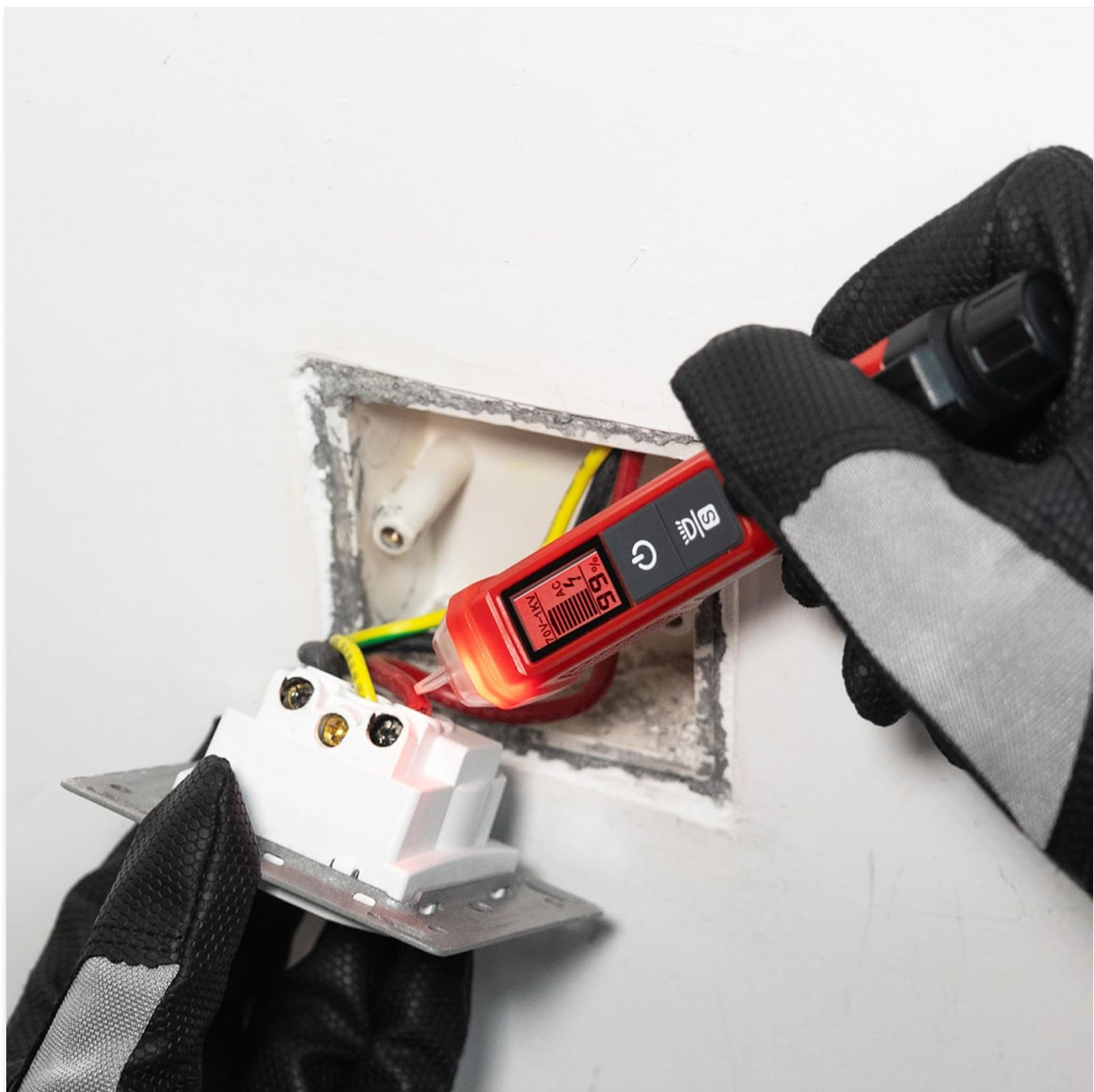
Image: The HT100s-R tester being used to detect voltage in an electrical outlet. The tip glows red, indicating voltage presence.
