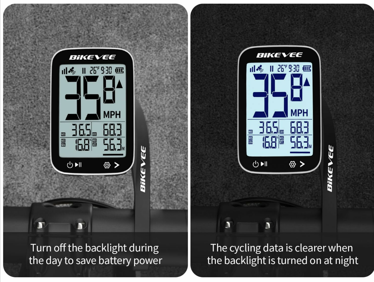
Image: The Bikevee cycling computer display showing the difference in visibility with the auto backlight off (left) and on (right), demonstrating improved clarity in low light.
