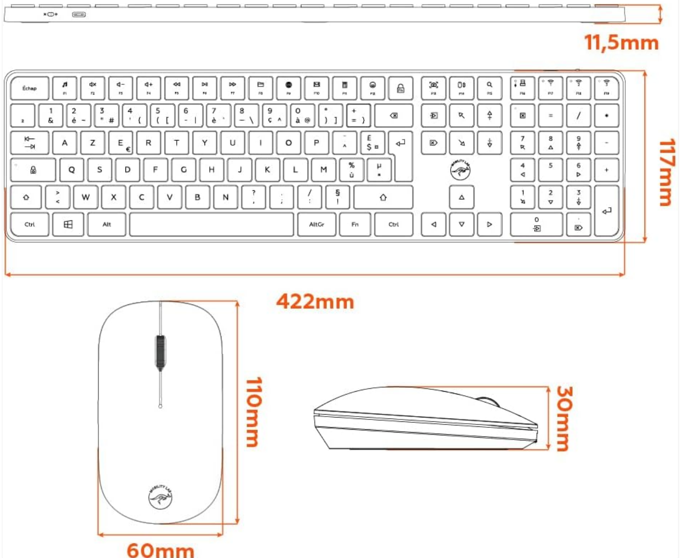
Image: A technical diagram illustrating the precise dimensions of both the keyboard and the mouse.
