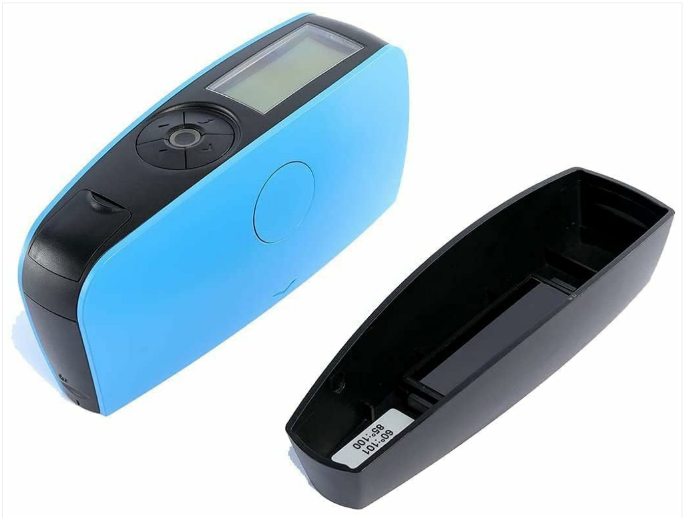
Figure 5: The gloss meter positioned next to its calibration plate.
