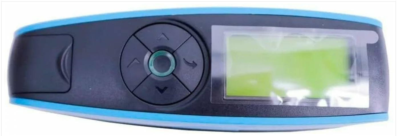
Figure 2: Top view of the gloss meter, highlighting the display and control buttons.
