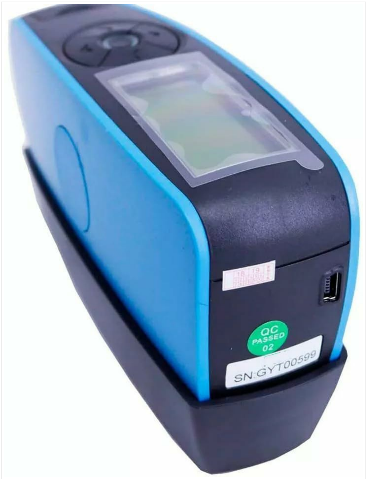
Figure 3: Side view of the gloss meter, showing the USB port for power supply and the product serial number.
