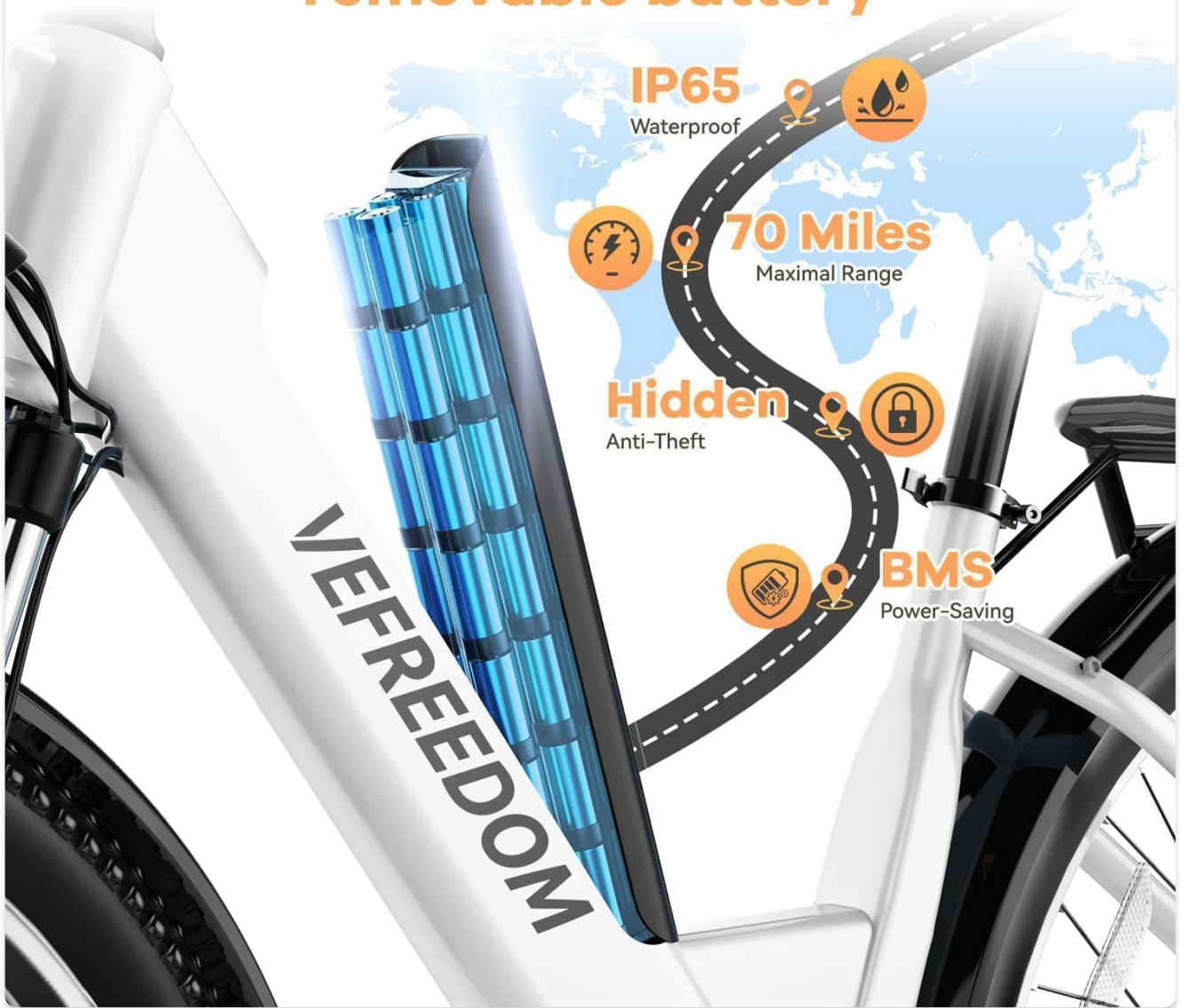
Image 5.4: Features of the removable battery, highlighting its range, waterproof rating, and anti-theft design.
