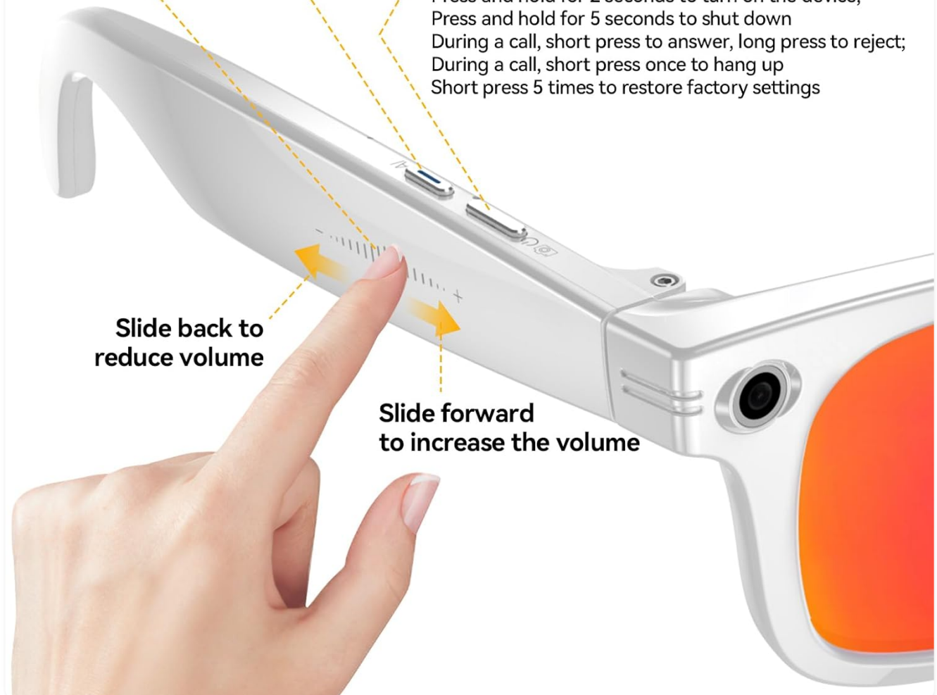
Figure 3: Button and Touchpad Controls.
