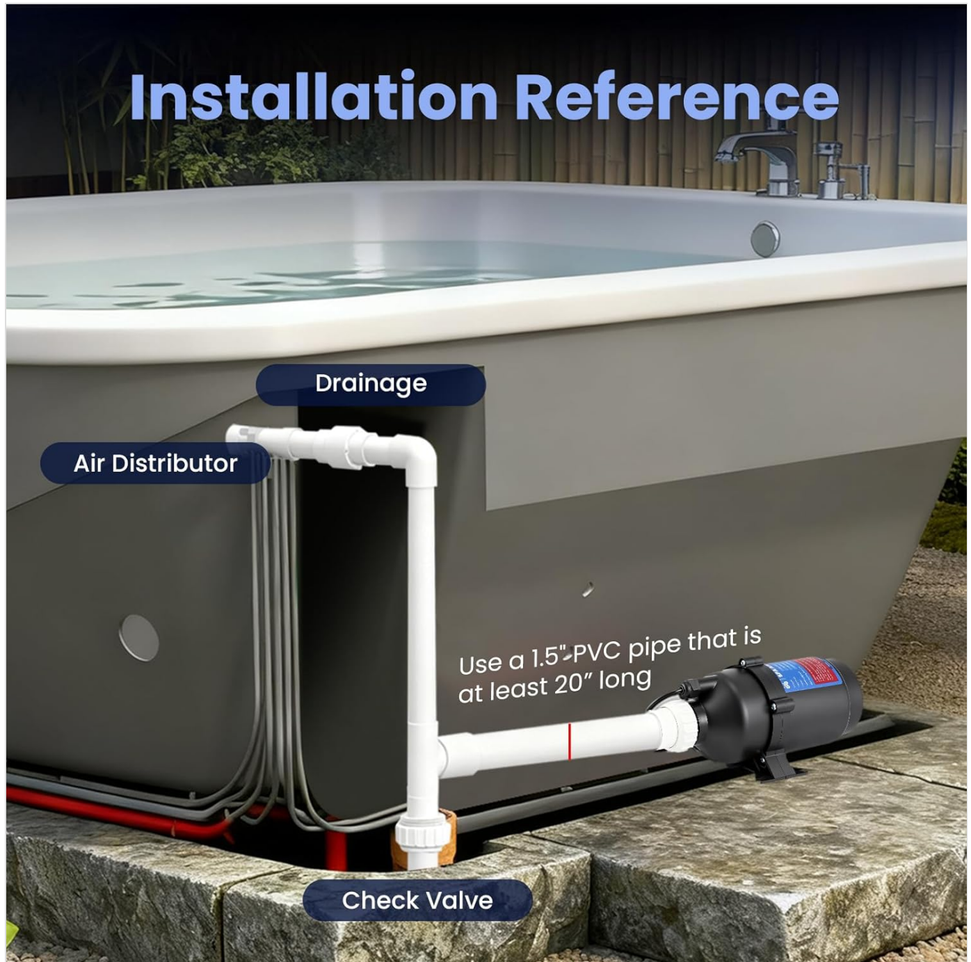
Image: An illustration showing the recommended installation of the SPA air blower with plumbing. It highlights the drainage, air distributor, and check valve, indicating the use of a 1.5-inch PVC pipe at least 20 inches long.
