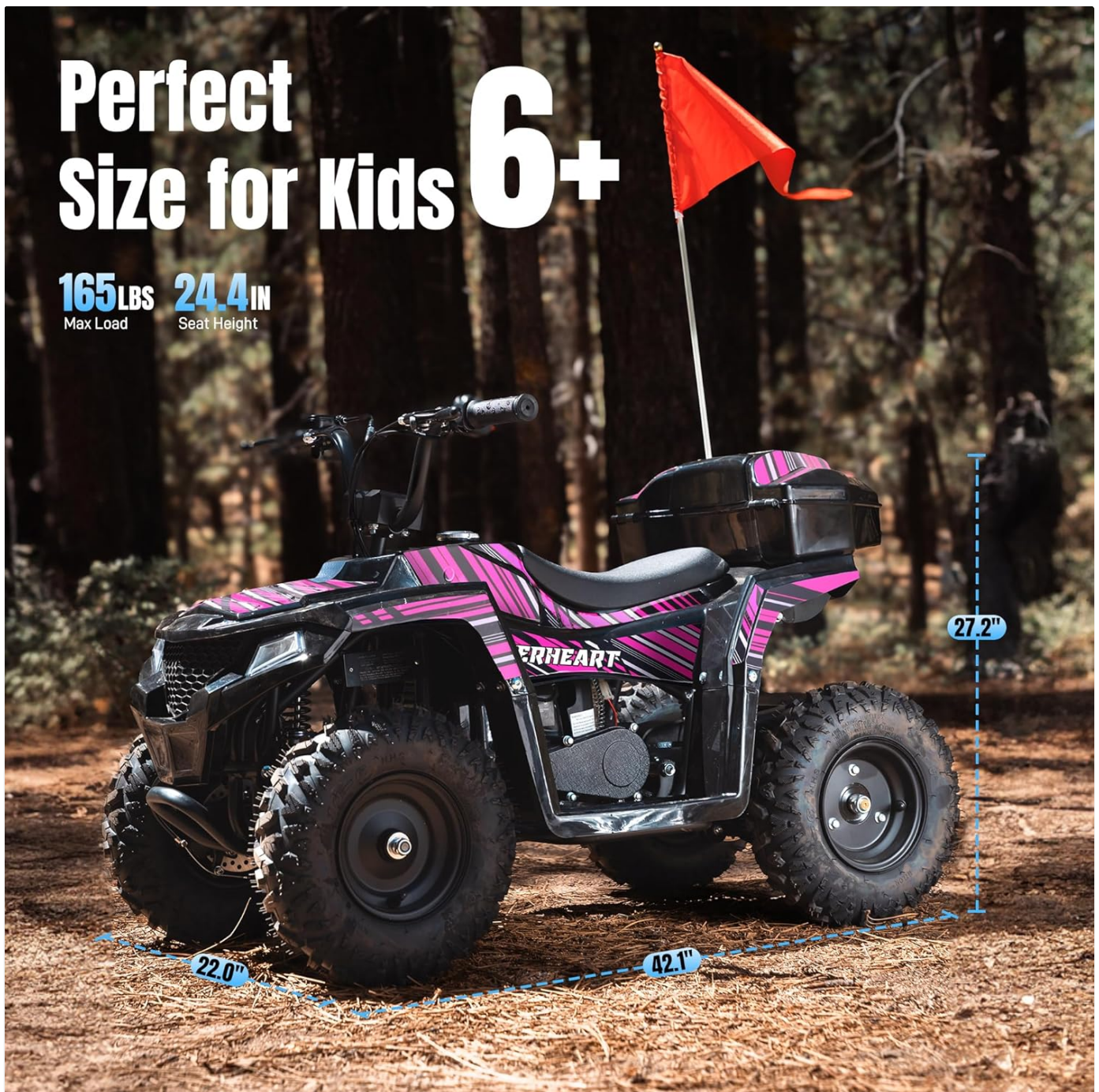
Figure 8.1: Key dimensions of the HOVER HEART XW-A19 ATV.
