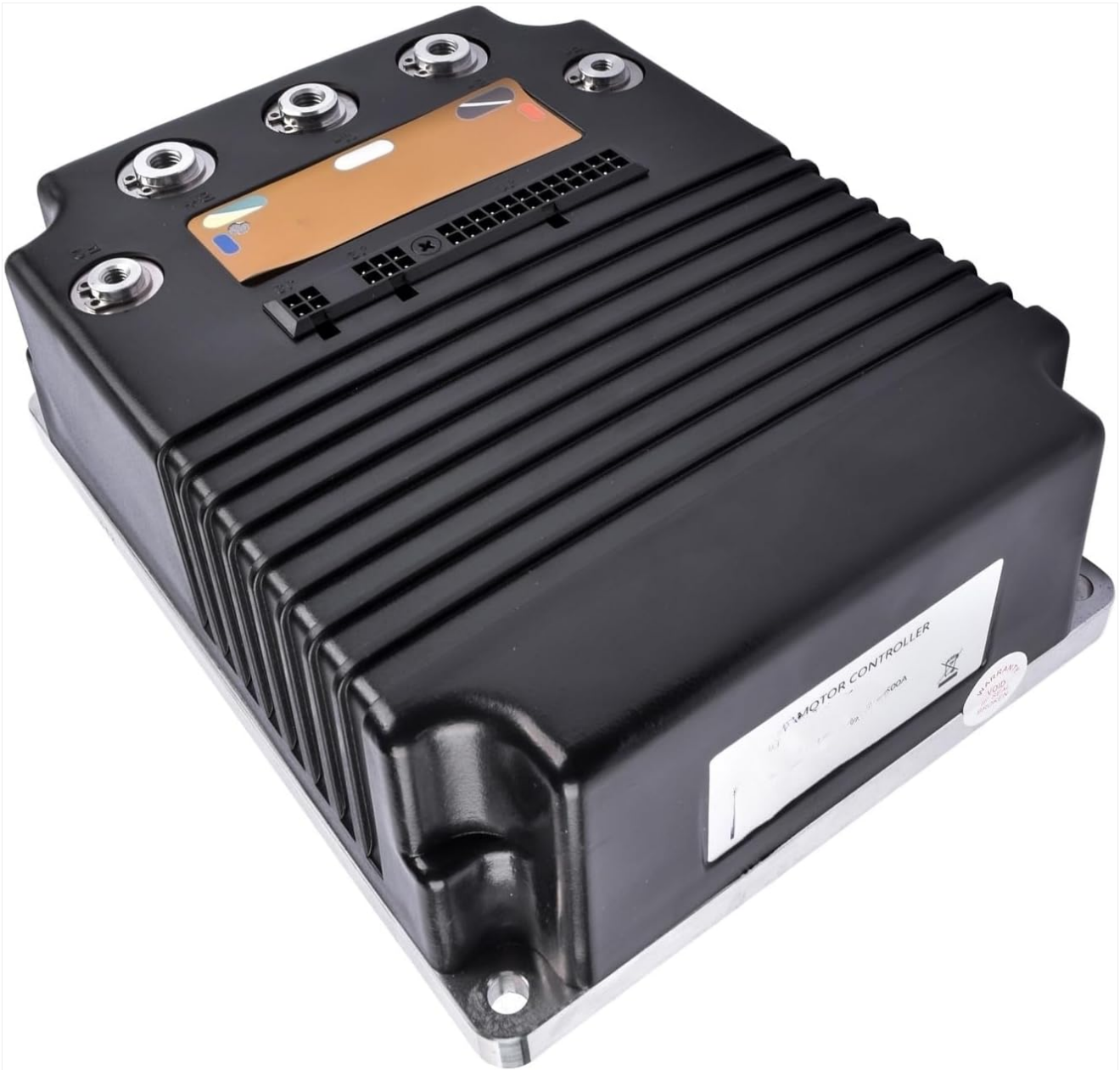
Figure 3.5: Side view of the controller, illustrating its compact form factor and the arrangement of the cooling fins on the top casing.
