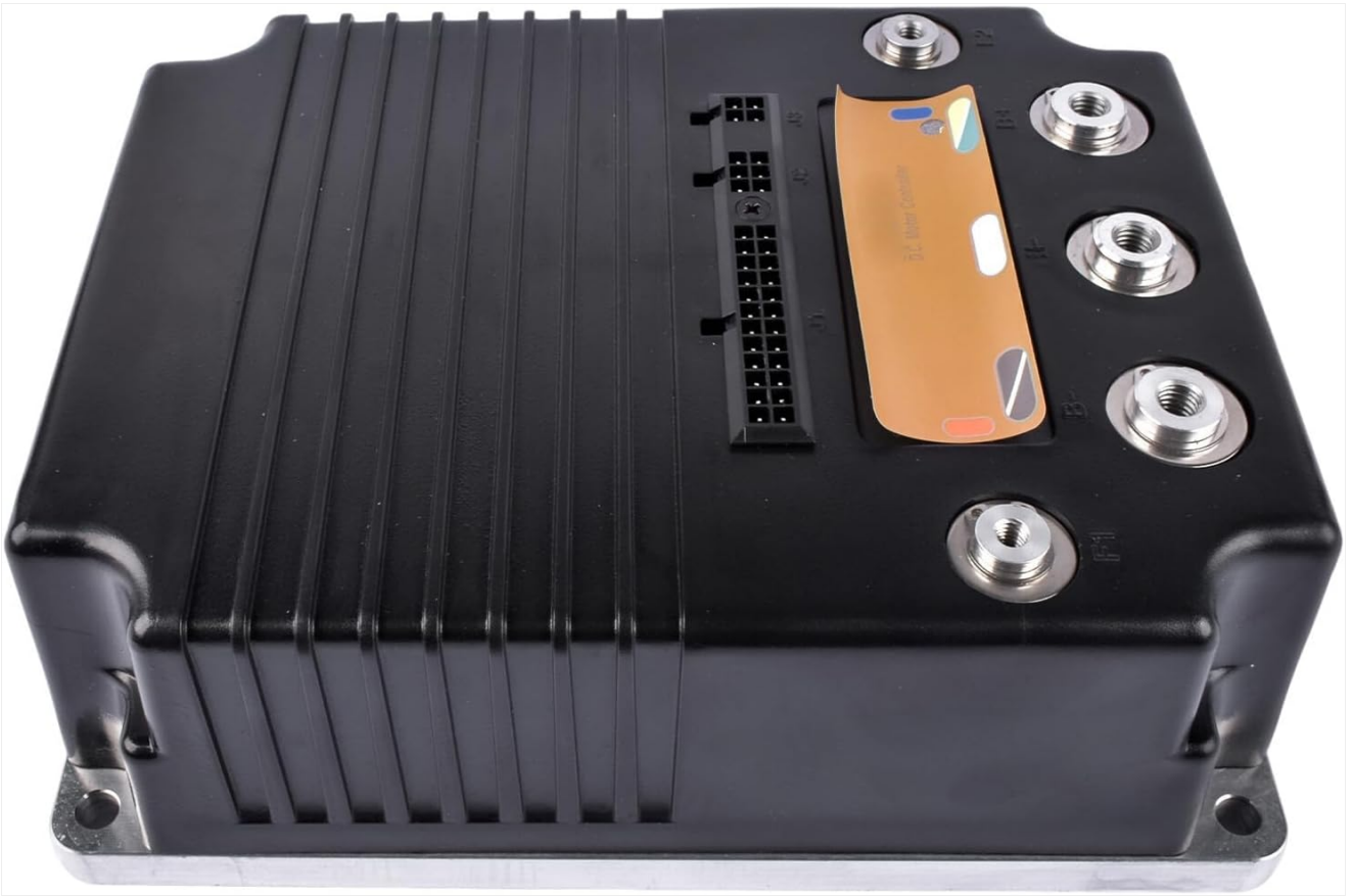
Figure 3.2: Angled view of the controller highlighting the various electrical connectors and terminals. The large terminals are for high-current connections, while the smaller multi-pin connectors are for control signals.
