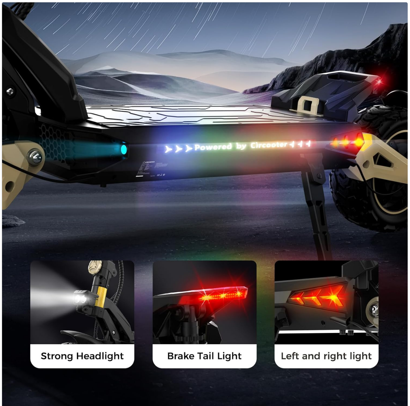
Image 5.2: The scooter's comprehensive lighting system, including a strong headlight, brake tail light, and left/right turn signals for improved safety and visibility.
