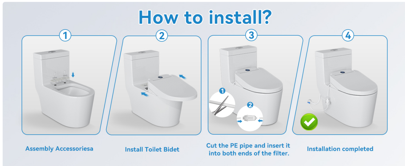
Image 5.2: Visual steps for installation: 1. Assembly Accessories, 2. Install Toilet Bidet, 3. Cut PE pipe and insert into filter, 4. Installation completed.
