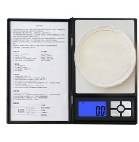
Image 5.3: Press the TARE button to zero the container's weight.
